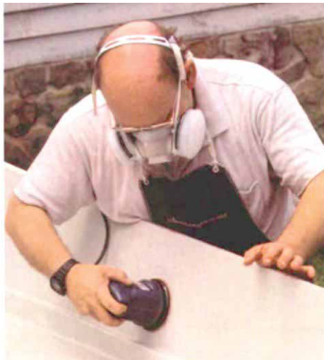
Half-face mask —These respirators are usually made of soft rubber or silicone and have replaceable filter cartridges.
