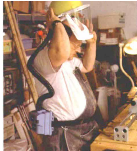
Full-face protection —Powered air-purifying respirators deliver a constant supply of filtered air.
