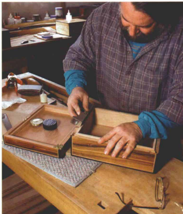
Careful with that bevel angle. It determines the rate the humididor loses humidity and receives fresh air. A humididor that is opened frequently should have a tighter fitting lid.
