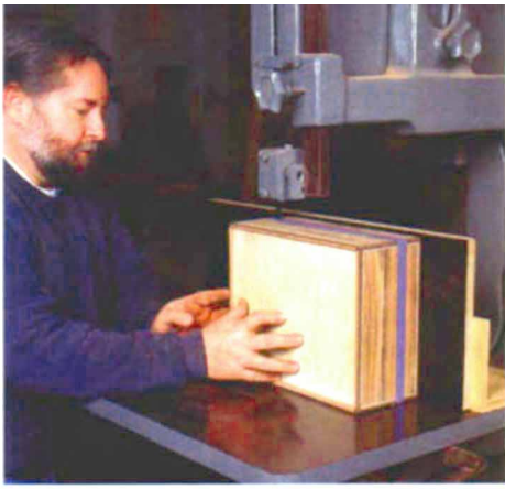
Saw the top off the box on a band-saw. Tape the entire saw line, and use a 1/2-in., 3-tpi blade to avoid breakout.
