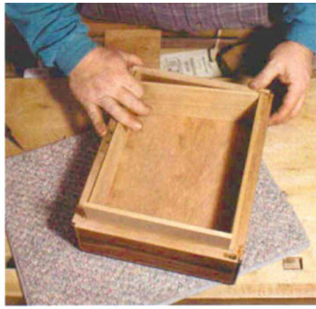
Gently press-fit lining around interior. When you season the humidifier, the lining will swell and lock itself in place.
