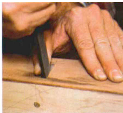
Square up the throat. A file fine-tunes the throat opening. To avoid tearout, cut on the push stroke only.
