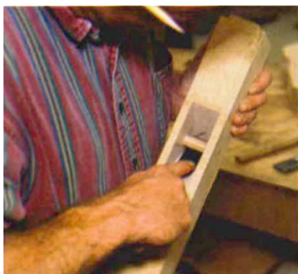
Cleanup —The author uses a chisel to make sure the plane iron ramp and the bevel in the slot are in line.
