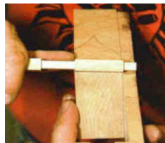
Cheeks should not pinch the cross-pin. When cut correctly, the cross-pin can rotate freely in holes bored through the cheeks.
