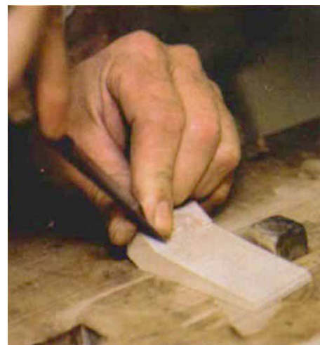
Center block offcut becomes the wedge. The author details the plane's wedge, which should be cut to a slope of 6^\circ to 8^\circ . A flat at the back presents a good surface for the hammer.
