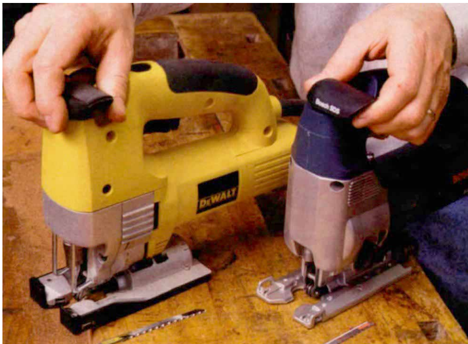
Two good ideas—DeWalt and Bosch (above) have very similar blade-releasing knobs located at the top of the tool. No tools are required.
