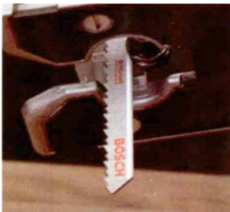
Typical blade guide —Most jigsaws come with a single, free-spinning guide located directly behind the blade. Some have quite a bit of play in them, which may allow the blade to deflect.
