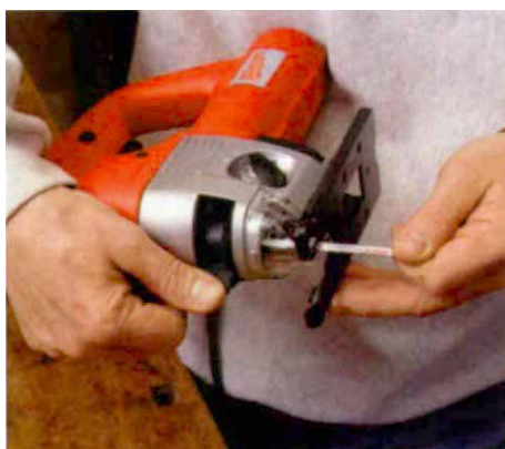
Two good ideas—DeWalt and Bosch (above) have very similar blade-releasing knobs located at the top of the tool. No tools are required.
