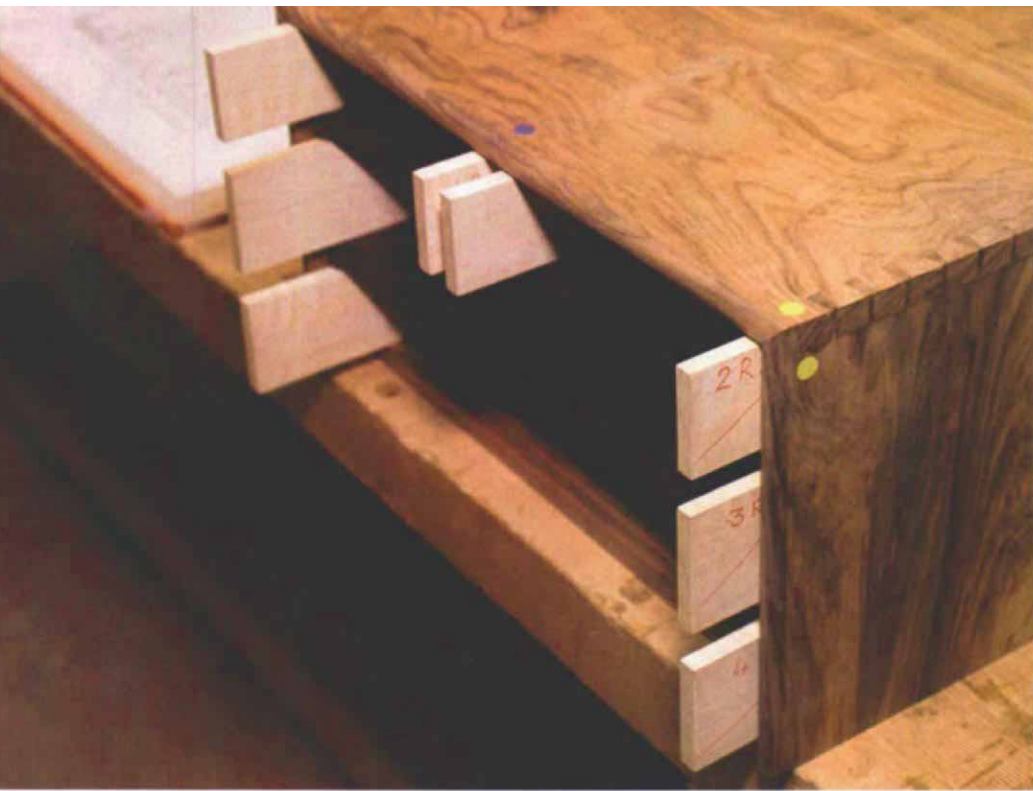
The sides have been fitted. The drawer backs are next. Colored dots at the corners of the case piece identify mating edges and indicate the front of the case.
