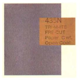
Aluminum oxide is a sharp and blocky mineral. It is the most common, all-purpose woodworking abrasive, and for good reason. It is the only abrasive mineral that fragments under the heat and pressure generated by sanding wood. This characteristic is called friability and is highly desirable. As you sand, aluminum oxide renews its cutting edges constantly, staying sharp and cutting much longer than other minerals.
