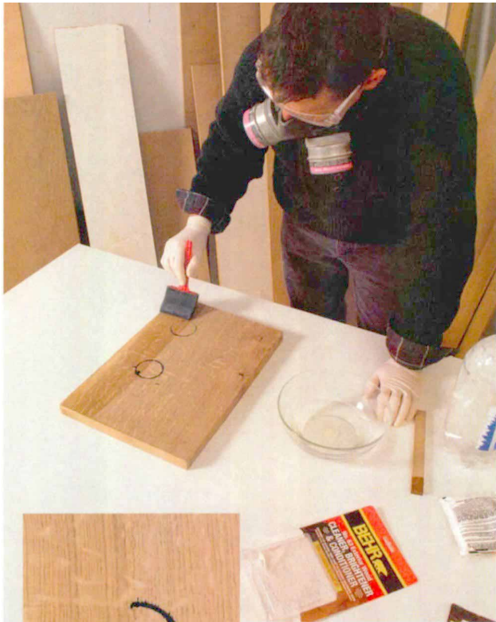
Oxalic acid removes the stain but not the color of the wood. The author used a deck brightener, which has oxalic acid as an active ingredient, on this piece of white oak.
