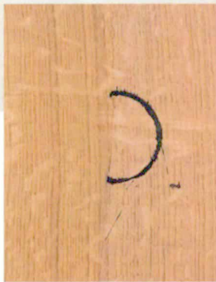
Oxalic acid removes the stain but not the color of the wood. The author used a deck brightener, which has oxalic acid as an active ingredient, on this piece of white oak.
