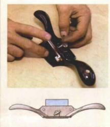
Flex the cutting edge of the blade. Tightening the thumbscrew on the back of the scraper body causes the blade to extend below the sole, allowing it to cut. The more the thumbscrew is tightened, the greater the blade projection.
