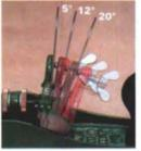
Change angle as scraper dulls. The author sets a fresh blade at about 5° off vertical. When it stops cutting, he adjusts it a few degrees forward. The blade can be adjusted until it reaches 20° before it needs reburnishing.
