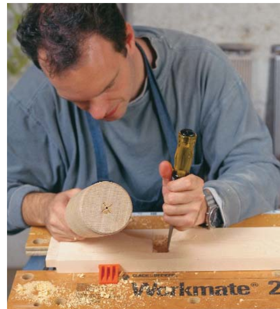
Gusset mortises—After boring holes on the drill press, the author cleans out the mortises by hand.
