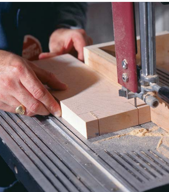
Tenons for the gussets, cut to size and shape with the bandsaw, pull the apron pieces tightly to the legs.
