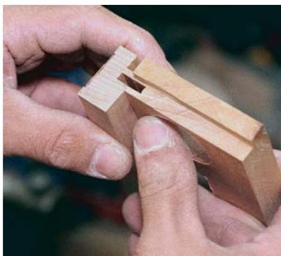
**Check the alignment (left).** The top of the middle shelf and the top of the front rail should be flush. The 1/4-in. groove accepts the bottom edge of the face panel.
