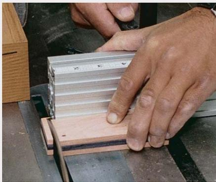
**2.** Plane the edges of each lamination square to the faces, and make sure the edges are free of glue. Cross-cut laminations into segments exactly  $\frac{1}{4}$  in. wide.
