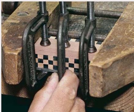
**3.** Arrange segments from alternating sandwiches. Glue and clamp them together. Apply pressure down, as well, onto a steel plate or something similar, to ensure even registration all the way across.
