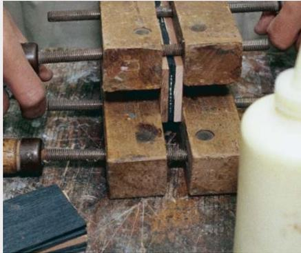
**1.** Prepare two "sandwiches" of material—one with a lighter wood in between two dark pieces, and the other just the opposite. Width and length aren't critical, but each layer of the laminations must be exactly  $\frac{1}{4}$  in. thick.
