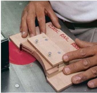
*A template and guide shape the top door rail. After bandsawing the curve in the rail to rough shape, the author routs it to finished shape.*
