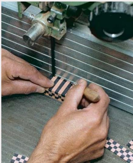
**4.** When the glue has cured, clean up and square the completed checkerboard blank. Bandsaw into  $\frac{1}{16}$ -in.-thick strips. Using a knife to pull the thin strips along on the out-feed side of the blade helps. Select the best pieces for the clock inlay.
