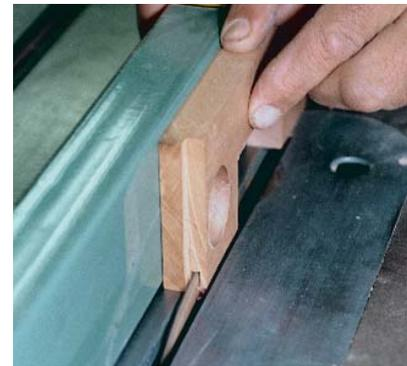
**Kerf front rail and middle shelf for a spline.** One pass with each piece over a standard-width blade is plenty. Then just plane the spline to fit.
