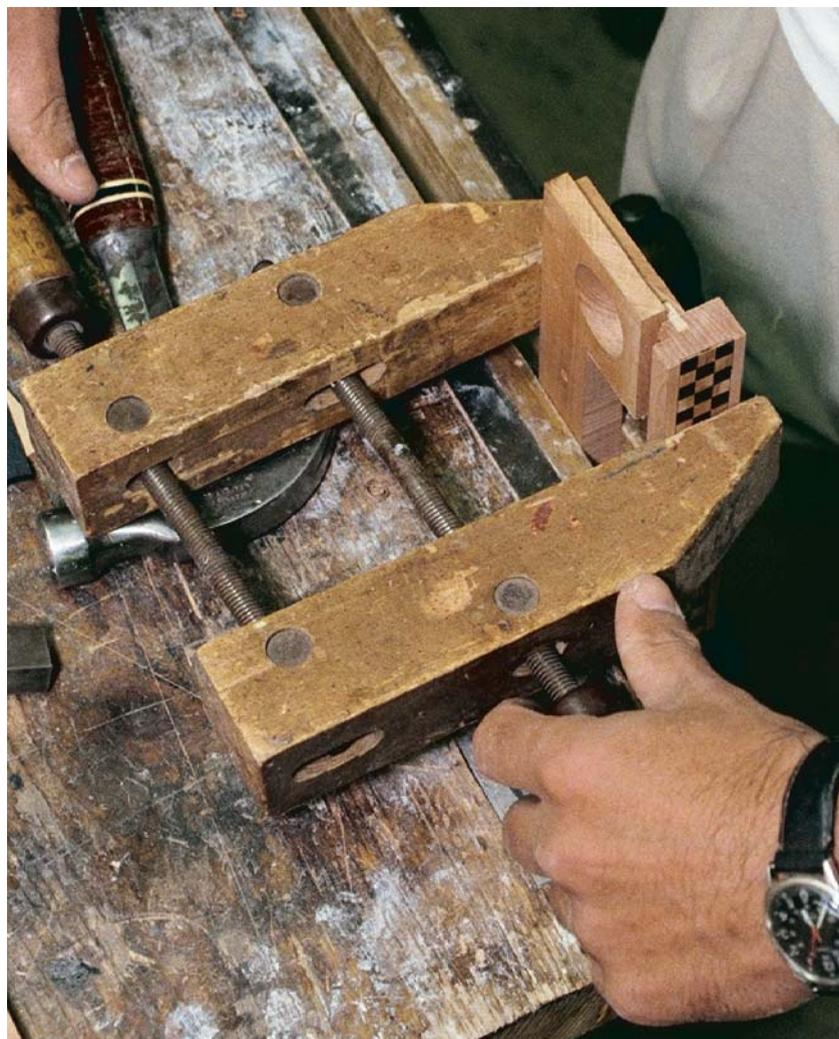
**Middle shelf and front rail are joined with a spline.** Hand screws provide plenty of clamping pressure, but be sure the front rail stays square to the shelf as pressure is applied.
