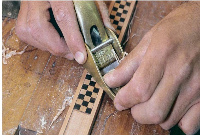
**Plane the front rail flush.** Using a sharp block plane is a quick way to bring the top and bottom edges of the front rail down to the level of the inlay.
