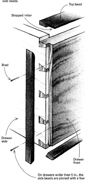
the side beads on drawers wider than about 5 in. are best secured with a few small brads in addition to glue. Drawers wider than 8 in. or so should not be cock beaded By setting the brads and filling the holes with a wax pencil of the same color as the cock bead, the holes are nearly invisible.
