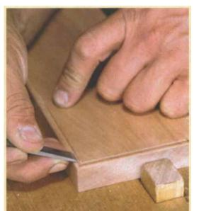
light cuts. The scratch beader can be both pushed and pulled. And it shapes wood across the grain nearly as well as it does with the grain.
