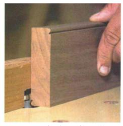
Router cuts beads quickly and consistently. When he has a lot of beading to cut, the author chooses the router. The only drawback is the limited availability of router bits with small profiles.
