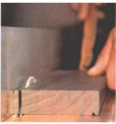
Beads are sawn offboth sides. The author leaves a little extra material next to the bead and then planes the bead to a precise thickness. A push stick is used to move the bead past the blade.
