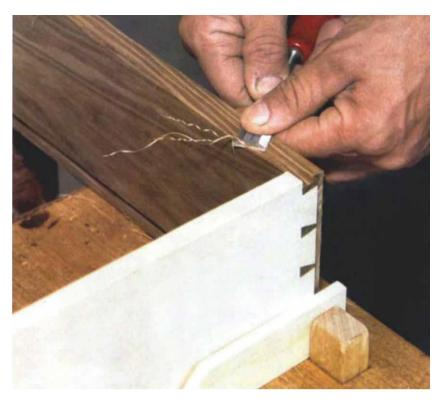
Clean up the back edge of the top rabbet. A knife or a chisel works well. Leaving this paper-thin buffer in place while routing prevents damage to the front edge of the drawer sides.
