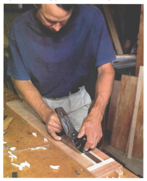
Plane strips of beading to thickness. A fixture consisting of three pieces of softwood glued and tacked to a piece of plywood holds the bead in place.
