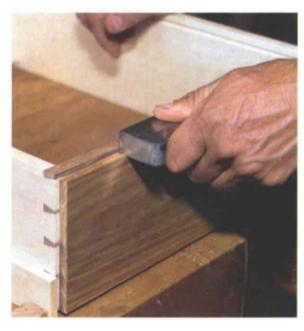
Bottom and side rabbets are cleaned up with a rabbet plane. The inside corners can be cleaned out with a chisel, if necessary.
