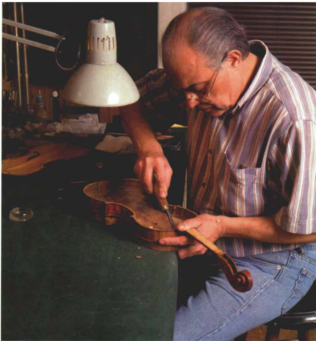
These instruments were designed to be taken apart. After removing the belly of this violin, Horacio Pineiro uses a gouge to carve away some of the end block that supports the neck.
