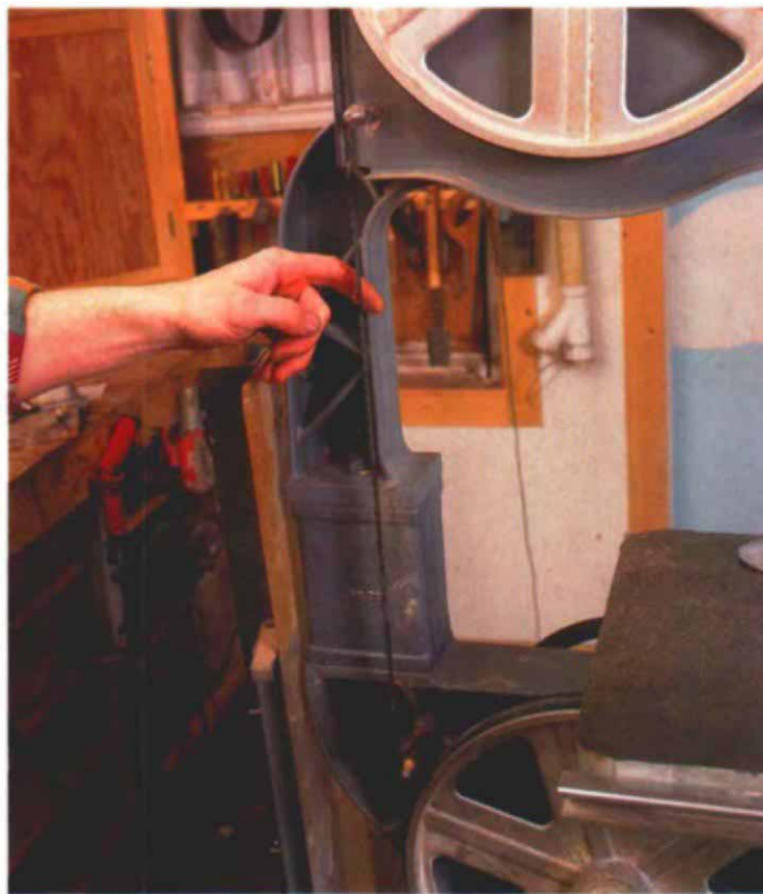
Pluck the blade to check the tension. Listen for a clear note, roughly an E on a bass guitar. The author replaces the blade guard after tensioning the blade.
