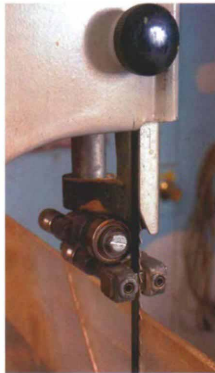
Raise the guide bar, and adjust the blocks and thrust bearing. Set the gap between guide blocks and blade to .002 in., and bring the thrust bearing in light contact with the back of the blade.
