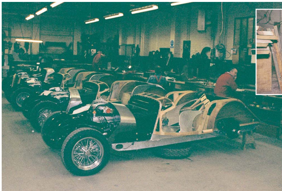
Frames start as slabs of European ash. A Morgan frame begins its journey on a band-saw in a shop adjoining the frame-assembly area (above). After frames are complete, cars move along for additional work (left).
