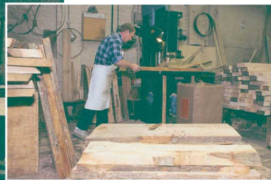
Frames start as slabs of European ash. A Morgan frame begins its journey on a band-saw in a shop adjoining the frame-assembly area (above). After frames are complete, cars move along for additional work (left).
