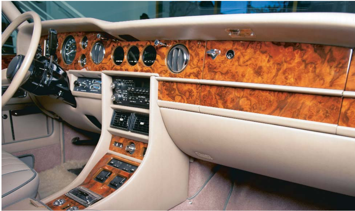
Woodworking art on wheels —Meticulously fitted and finished, this dashboard and console in burl walnut veneer is a characteristic detail of the Rolls-Royce, this one in a busy Connecticut showroom.
