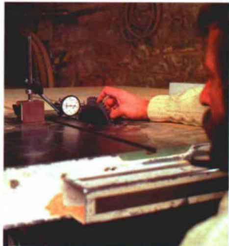
Measuring runout indicates flatness. Blades in this evaluation had runout of between .003 in. and .005 in.
