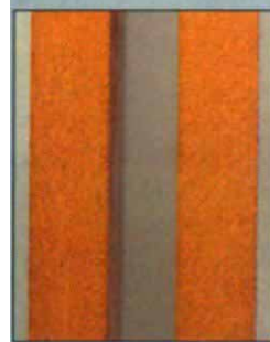
Medium-density fiberboard cuts smoothly. Differences in blade performance were not significant when it came to scoring, or sawmarks, left behind by blades in the sawn face of MDF (photo at left). That is also the case in how blades performed on the bottom edges of MDF samples (bottom photo).
