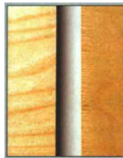
The bottom edge of the plywood shows the difference. The crosscut sample at left is representative of the best blade performance. The sample at right is an example of blades that made acceptable cuts.
