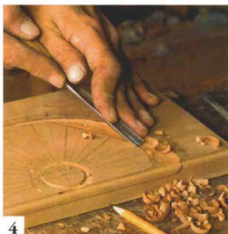
4 Shape the fan background across the grain. Developing the S-shaped surface with mostly cross-grain cutting gives greater control over the tool.
