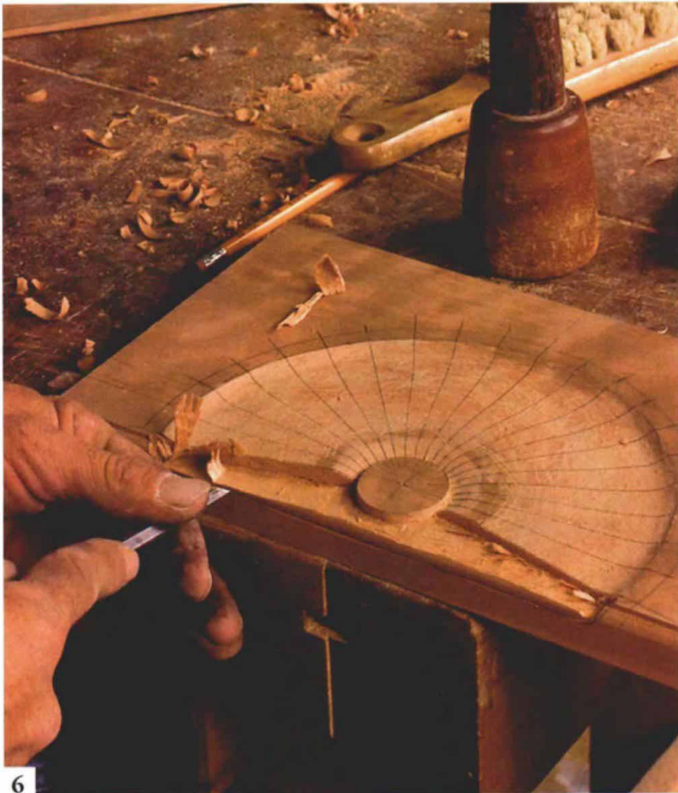
Use a bench chisel to remove the waste below the fan. This surface provides the transition from the carved drawer to the case rail.
