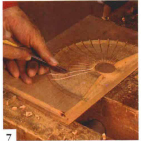
A V-parting tool is used to define the rays. Because the surface is S-shaped, wood grain can change direction. Take care not to run tools against the grain, which could cause tearout.
