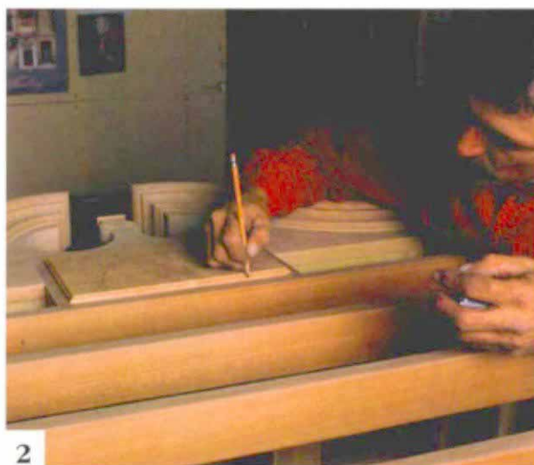
2 A scribe line marks the depth of the carved surface below the fan. This area forms the transition between the fan and the case rail.
