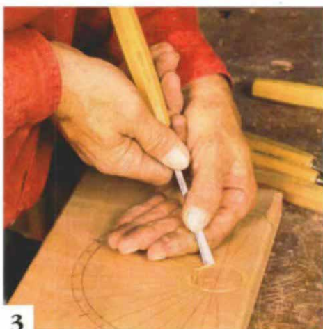
3 To prevent wood from splintering into the hub surface, outline this area with carving tools.
