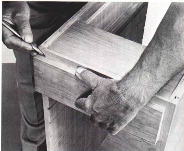
For a perfect fit, Frid fits the drawer parts individually before assembling them, first trimming the drawer front to a tight fit in the carcass opening. If the drawer front's length can't be scribed from inside the case, mark it directly from outside.
