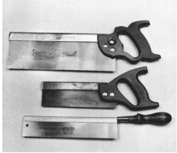
The fine teeth and thin blade stiffened by a brass or steel back make the backsaw an ideal joint-cutting tool. Backsaws are of two types; the larger are called tenon saws, the smaller are dovetail saws. Shown above are a 12-in. English-made brass-backed tenon saw, an 8-in. dovetail saw, and a 7-in. dovetail saw with the straight turned handle preferred by some craftsmen.
