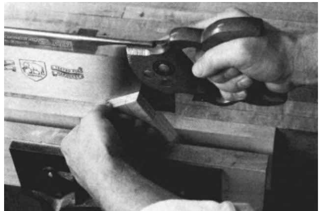
To saw tenon cheeks, mount the workpiece in the vise at about a 60° angle as shown above and start the cut at the edge of the piece opposite you. Carry the kerf over, and without lifting the saw out of the cut, pivot it toward you and saw down the cheek line until you reach the shoulder. Reverse the workpiece in the vise and saw down to the other shoulder line.
