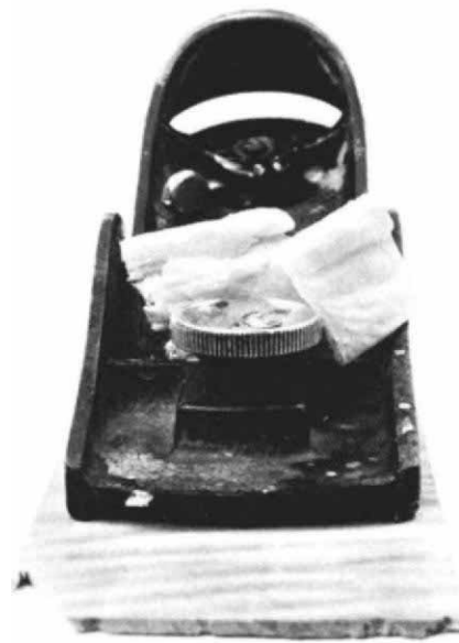
This tuned block plane easily smooths a curly maple strip that showed severe tearout after a pass over the jointer.
