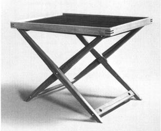
The taper in the legs of this stool cuts down weight, leaves the wood where it's needed, and allows the stool to close up to a snug 1¾ in. T-nuts in the stretchers allow disassembly. You don't have to store this stool in the closet when you're not sitting on it—make a tray that converts it into an occasional table or server, as shown above.
