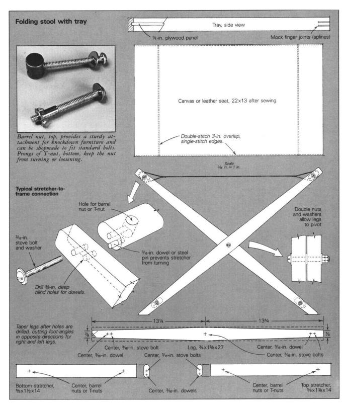
for the bolts and dowels. The stool is now ready to be assembled, but first chamfer all the edges with a router or a plane, then sand and finish the pieces.
