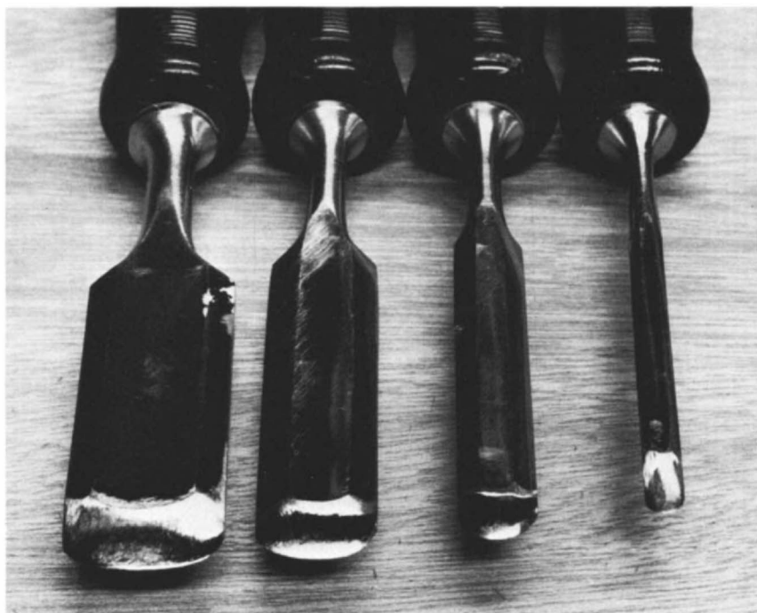
For doing the work of many carving gouges—roughing-out relieved areas and smoothing convex surfaces—Schramm made this set of round-nose chisels by re-grinding standard butt chisels. The long hollow-ground bevels are especially well suited for carving.
