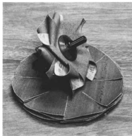
To make honing quick and tidy, Schramm constructed this rotary strop (above left) from plywood and leather. He mounts it in his drill press and charges the surface with white rouge, a simple arrangement for keeping a razor-edge on all his tools, without the mess made by oilstones. Pinwheel sander (above right), when chucked in lathe or drill press, is good for finishing contoured furniture parts like cabriole legs.
