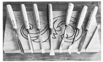
Relief carving tools (from left): V-tool for outlining, three gouges for general shaping, long bent grounder for backgrounds, spoon gouge, and flat or firmer gouge. The blank is butternut, held to the bench by a long screw from underneath.
