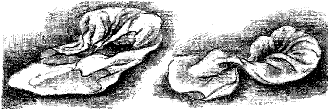
A square of cotton cloth is wrapped around a wad of cotton batting a little smaller than a tennis ball. Finishing material is poured in, and the cloth is folded and twisted around. Hand pressure controls the flow onto the wood.
