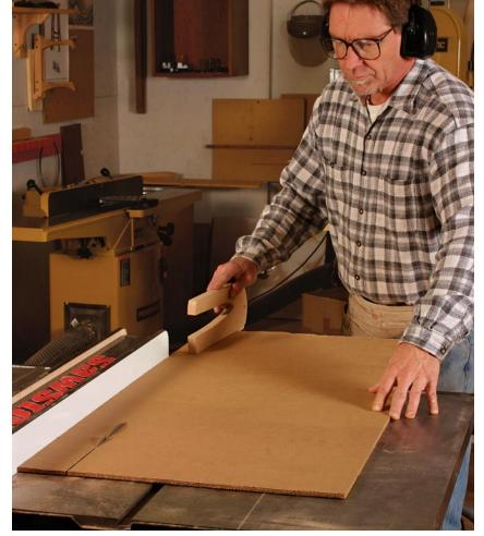
**The material cuts easily.** Components for a full-scale table model can be made in minutes. Just slice up cardboard parts on the tablesaw and glue them together.
