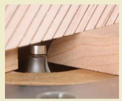
**Round off the bottom corner.** Flip the top over and slightly ease the bottom corner of the edge.
