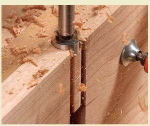
**Drill where you can.** The swing arm has sockets at both edges that need to be scooped out. Do this at the drill press with a <sup>3</sup>/<sub>4</sub>-in. Forstner bit, using the same fence and stop block setup as before.
