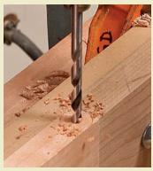
**Drill for the pin.** For the joint to work without binding, this hole must be straight and parallel to the end grain. Use a slow feed rate and drill halfway from each edge.
