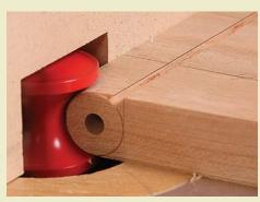
**Round over the end.** Gochnour uses a %-in.-radius bullnose bit to form the rounded knuckle in one pass. This allows the joint to swing open and closed.
