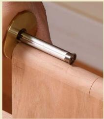
**Transfer the knuckles.** After making a small tick with a knife (left), use a marking gauge to complete the layout (right). To do this, put the gauge's blade in the tick mark, set the fence against the board's edge, lock it, and scribe. Repeat for each tick mark.
