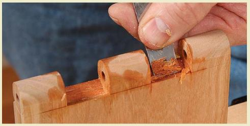
**Handwork where you can't drill.** Use a chisel, bevel down, to scoop out the area between knuckles. Gochnour moistens the fibers with mineral spirits—an old carver's trick—to soften them and get tearout-free results.
