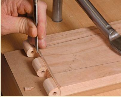
**Straight shoulder for now.** After defining the knuckles with a backsaw and removing the waste with a coping saw, pare down to the stop. A straight shoulder helps when you transfer the knuckles to the mating piece.
