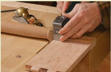
**Trim it flush.** After gluing the swing arm to the gate leg, trim the notch's cheek level with the arm.
