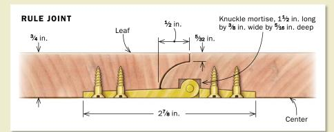
can cut the hollow between the knuckles. On the edges of the swing arm, use a 3/4-in. Forstner bit and the same fence and stop block setup as for the hinge-pin hole. Between knuckles, you'll have to scoop out the waste with a chisel, used bevel down. Check your progress with a 3/4-in.-dia. dowel. When it sits flush with the rounded end of the knuckles, you're done.
