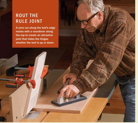
**Press down hard.** It's critical that the routed edges of both sides of the joint be uniform and smooth, so use push pads and a featherboard to keep downward pressure on the tabletop and leaves when feeding them through the bit.
