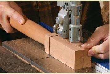
**Notch the leg.** This allows the leg to fit under the inside, continuous apron. Cut the shoulder at the tablesaw, then the cheek at the bandsaw.
