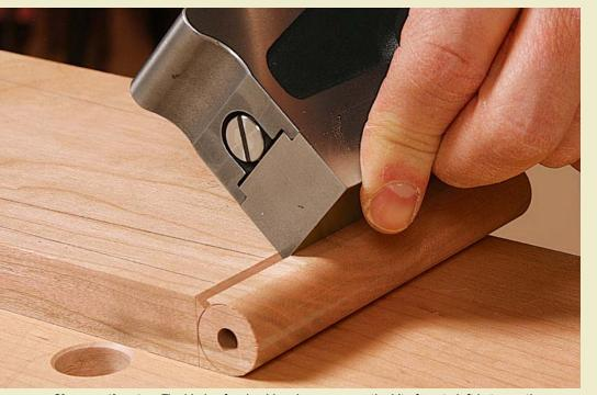
**Clean up the stop.** The blade of a shoulder plane removes the bit of waste left between the rounded end and the stop cut into the face.
