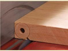
**Lay out and cut the stop.** Use a marking gauge to scribe a line across the board's edge and across its outside face (left). Then, with the blade angled 45°, cut a kerf on the outside face at this cut line. Repeat for the other half of the joint to create a 90° stop.
