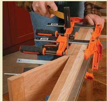
**Glue on the fixed arm.** Spread glue on both the tenon and the inside face of the fixed arm (left). Leave it in the clamps for several hours. Attach the gate leg (above). Put the two halves of the knuckle joint together and then drive a <sup>1</sup>/<sub>4</sub>-in.-dia. steel rod into the hole. Gochnour grinds a chamfer on the ends of the rod.
