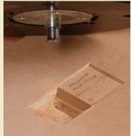
Add a spacer for the barrel mortise. The spacer snaps into the jig (left), and provides a bearing surface for a bushing, allowing you to rout the narrow mortise for the hinge barrel.
