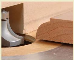
**Two bits make the joint.** Rout a cove into the underside of the leaf, using a %-in. radius cove bit and leaving a %-in. flat on the edge (left). Then, put a %-in. roundover bit in the router table and rout both edges of the center section of the tabletop (right).
