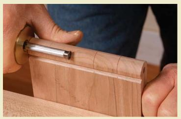
**Get symmetrical knuckles with a gauge.** Lay out the knuckles from both edges of the board. Two settings will produce four lines and five knuckles.
