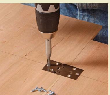
Drill for the screws. Use a Vix self-centering bit to ensure that the pilot holes are centered in the leaf's screw holes. Gochnour saves the hinge's brass screws until after the table is finished. Steel screws the same size are more durable and can be driven in and out during construction without damage.
