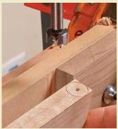
Mark the center and circumference. A <sup>3</sup>/<sub>4</sub>-in.-dia. Forstner bit does both at once. Use scrap to dial in the location of the fence and stop block so that the bit's cutters hit the end and two sides.
