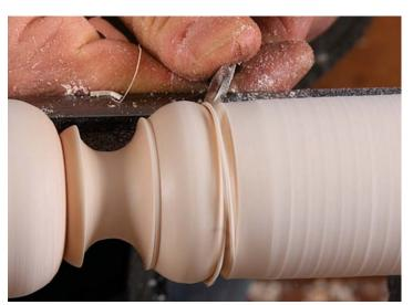
Then the bead and V-groove. With a few light skew cuts, the bead finishes taking shape, and a clean V-groove is formed next to it.
