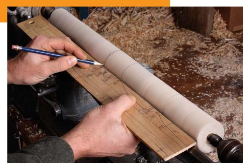
Lay out the largest parts. Galbert marks each feature using a full-size template (above). In this case it's a Windsor chair leg. Using a parting tool and calipers, establish the diameters of the thickest parts (right).
