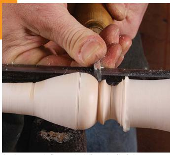
**Cut deep coves before nearby delicate details.** Galbert forms the mushroom cap after the deep excavating cuts that shape the cove—avoiding the potential harm they could do to a finished detail.
