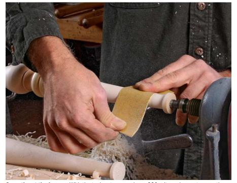
Smooth out the bumps. With the tool rest removed, use 220-grit sandpaper to smooth out leftover tool marks. Sanding has an added benefit—the texture it leaves behind helps the finish adhere better.
