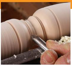
**Detail work.** With all the rough shapes established, use the pattern to mark the details (left). Part them to diameter, then slow the speed to 1,000 rpm and use a spindle gouge to start shaping the details, starting with the cove (above).
