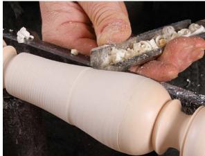
**Now shape the neck.** Leaving it thick kept vibration to a minimum while shaping the small details. Now use a roughing gouge to trim down and shape the neck, and finish it off with a skew chisel.
