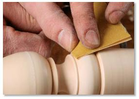
Clean up near details. Fold a piece of sandpaper to sand right up to the details without rounding corners.
