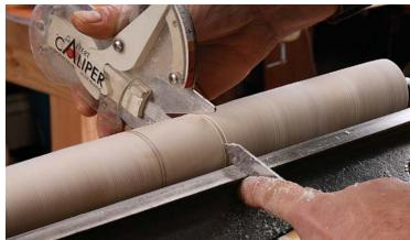
Then rough out the overall shape. Begin to shape the large features with the roughing gouge. Use the same tool to remove the waste around the smaller-diameter parts. This step gets excess material out of the way, making the next step of parting easier.
