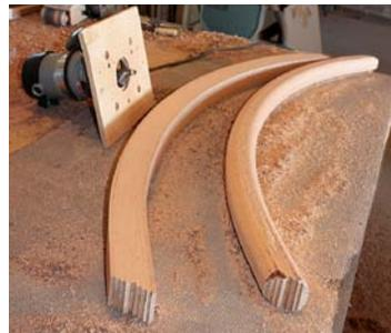
All the vertical elements get shaped with a roundover bit in either a handheld router or on a router table. Before routing the bent-laminated pieces, Pulver uses a power plane to flatten the surface and roughly round the corners on the convex side.
