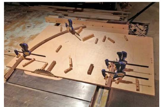
For crosscutting, a plywood jig festooned with clamping blocks holds the vertical elements exactly as they'll be in the table. A 4-in.-wide spacer against the fence permits uncut ends to overhang the jig.
