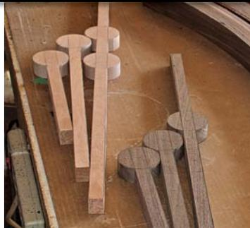
The curved elements are bent laminations made with 3/4-in.-thick solid-wood plies clamped on a particleboard form. The lollipop-shaped elements are laid out on a plank and bandsawn to shape.
