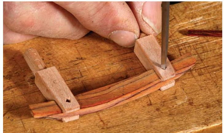
**Follow with the chisel.** Use a  $\frac{1}{16}$ -in. chisel to chop the miniature mortises. To remove waste during chiseling, Day redrills with the  $\frac{1}{16}$ -in. bit.
