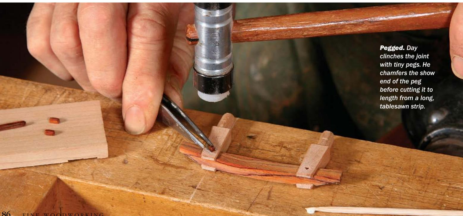
**Pegged.** Day clinches the joint with tiny pegs. He chamfers the show end of the peg before cutting it to length from a long, tablesawn strip.
