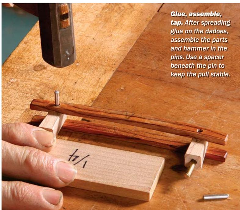
**Glue, assemble, tap.** After spreading glue on the dadoes, assemble the parts and hammer in the pins. Use a spacer beneath the pin to keep the pull stable.
