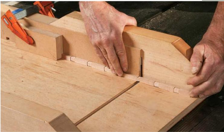
**One stick, many posts.** Day mills a long workpiece that will yield a batch of posts. He roughs out the tenons on the posts by dadoing across all four sides.
