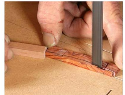
**Tiny dados.** With the bar blanks still milled square, use a crosscut sled with a stop block to cut the pairs of dados at both ends (left). Use a chisel to chop the outside shoulder of the dado to match the taper of the post (above left). Then carefully bandsaw the inner curve (above right), and fair the curve with files and sandpaper.
