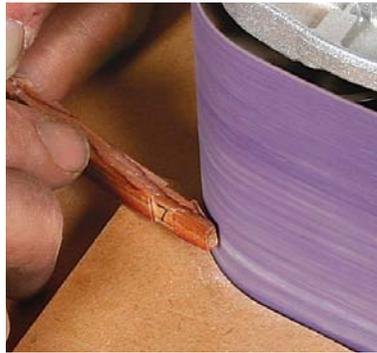
**Scoop with the sander.** Day uses his belt sander, clamped on its side and fitted with a shopmade "table," to shape the scooped sections at both ends of the bar.
