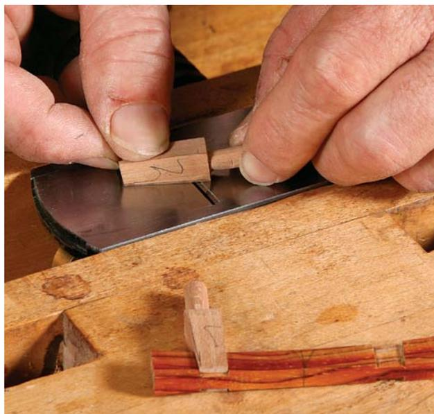
**Fitting the posts to the bar.** Using a block plane inverted in his vise as a finger-powered jointer, Day angles the outer face of the post to fit the dadoes in the bar.
