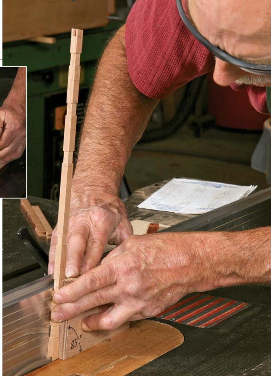
**Slot for the bar.** After crosscutting the ends of the workpiece at an 85° angle, use an angled guide block to cut the slot. Then cut a post blank from each end of the workpiece and repeat the process.
