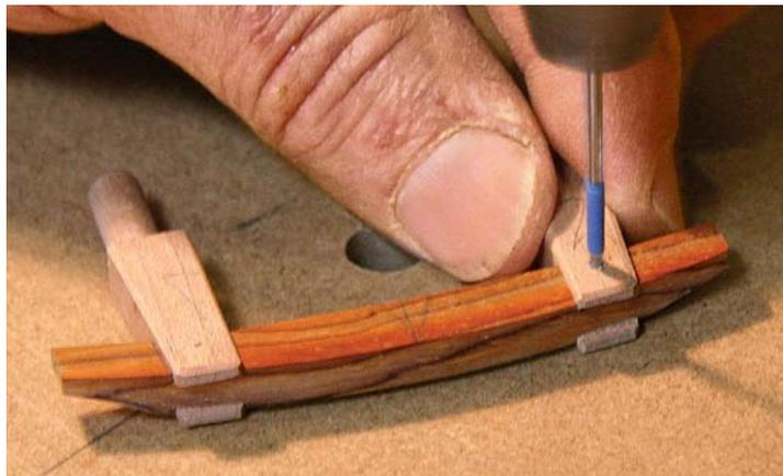
**Drilling for diamonds.** Before chiseling out the diamond-shaped mortise for the plug, drill a  $\frac{1}{16}$ -in.-dia. hole through the post and into the bar.
