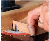
Cut the short leg of the L. The first step in creating the strap's L-shaped back is removing material at the top. Peart makes passes with a core-box router bit.
