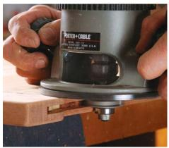
**More mortises.** When the breadboard ends come out of clamps, rout the mortise for the ebony splines that visually connect the ends to the panel. Peart uses a bearing-guided slot-cutter.
