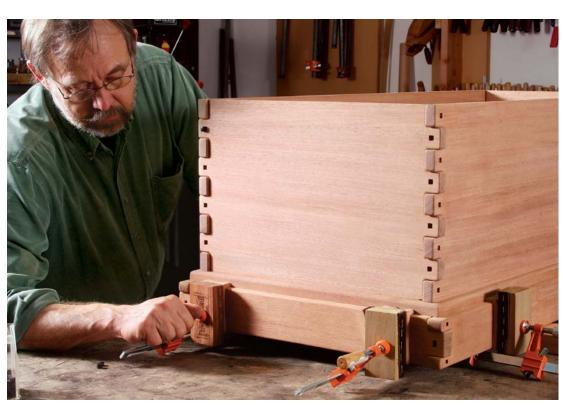
Glue the straps in place. No screws are used to secure the L-shaped brackets.
