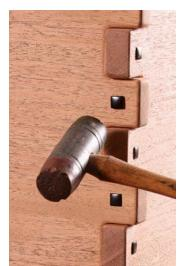
**Install the plugs.** After shaping and fitting the plugs, dab with glue and tap home with a small plasticheaded mallet.
