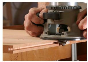
**Slots first.** To hold the splines that align the breadboard ends, Peart routs slots in the end grain of the lid panel and in the mating edges of the breadboard ends.
