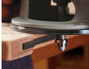
**Fit the spline.** Bandsaw the inner edge of the spline to roughly fit the stepped contour of the mortise bottom. With the spline pressed into place, pencil a line for bandsawing the outer edge to shape. Trim the excess, but leave it proud. A spiral bit with an extralarge bearing follows the irregular surface where the panel meets the breadboard end, trimming the spline uniformly proud.
