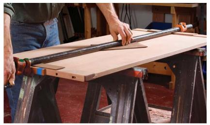
**On go the ends.** One clamp provides the pressure to secure both breadboard ends. To avoid problems with wood movement, apply glue along the whole length of the slot in the lid panel, but only the center few inches of the slot in the breadboard ends.
