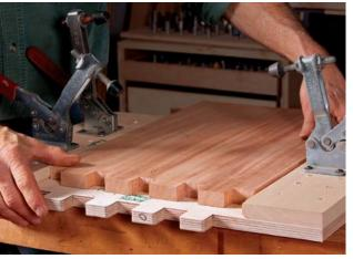
Rout the fingers. After removing the bulk of the waste with a jigsaw, clamp the workpiece into the template jig and use a 1/4-in.-dia. flush-trimming bit to complete the finger pattern on the end of each piece.
