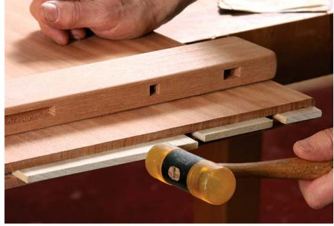
**Multiple splines make room for screws.** Peart leaves ½-in. gaps between the splines to provide clearance for the long screws that will help hold the breadboard end in place.
