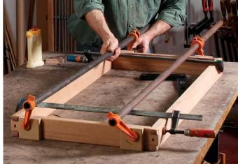
Build the base. Cut the large finger joints at the tablesaw with a dado set, then assemble the base like the case itself: Glue and screw the opposing corners, then bring the two halves together.
