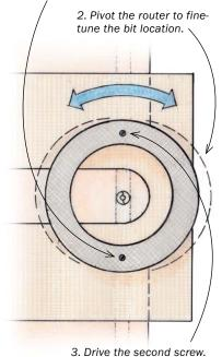
Line up the router with the cut. The
