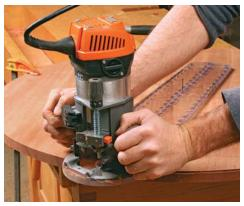
Rout at full depth. Lock the router at full cutting depth, but again raise it up before turning it on. Lower it gradually to full depth as you push forward, moving counter clockwise.
