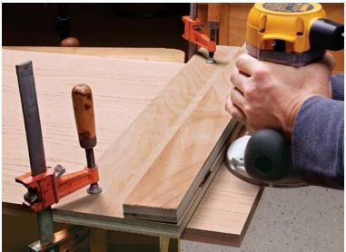
Flip and go. Now flip up the hinged section, and rout along the fence. The cut will line up precisely with the layout line. In case the router base is not concentric with the bit, keep the same point in contact with the fence as you rout.
