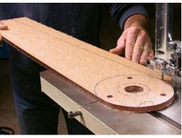
**Bandsaw the perimeter.** Polycarbonate saws and drills nicely. Smooth rough edges with a sanding block.
