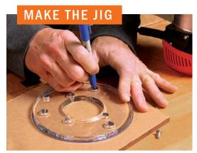
Lay it out and drill. Use the router's baseplate to locate the attachment holes on the jig, plus the 1½-in.-dia. center hole for the bit. Leave the protective paper on the polycarbonate for now.
