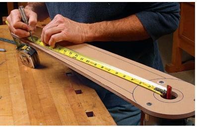
**Mount the router to lay out the pivot points.** Use a scratch awl, and turn the bit slightly each time, so a cutter is aligned with the mark you are making. The three lines merely space out the pivot points on the jig, so you have room to label them all clearly.
