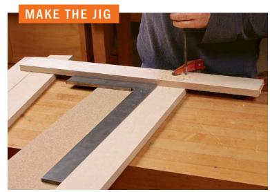
**Attach the first rail.** Use a large square to line up the first rail with the fence, clamping it in place before drilling holes and screwing it down.
