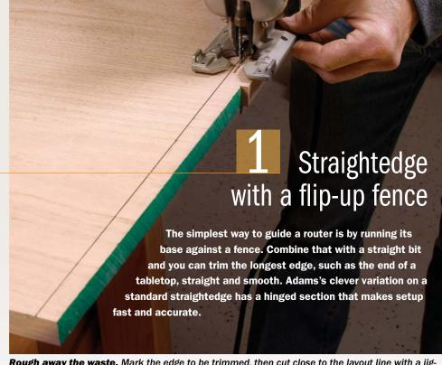
**Rough away the waste.** Mark the edge to be trimmed, then cut close to the layout line with a jig-saw or circular saw. Leave  $\frac{1}{8}$  in. or less for the router to trim.
