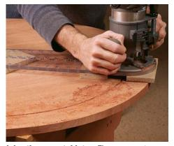
Inlay the same tabletop. The same router can plow a perfect inlay groove near the perimeter. Taped-on blocks hold the pivot and jig on the top of the table.
