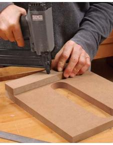
**Attach a fence.** Glue and nail it in line with the edge of the base.
