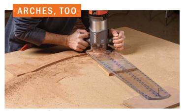
Make a workstation. To rout smooth curved templates, use carpet tape to attach the workpiece to a sacrificial panel of some kind. Attach blocks to the panel and jig as shown to keep it level with the workpiece. Set the bit to rout just slightly into the panel below.
