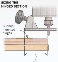
Hinged section matches distance between edge of base and bit.
