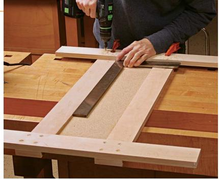
**Now add the second fence.** Be sure that the spacer is tight against both rails, and that the fence goes on square. Again, clamp before drilling and driving screws.
