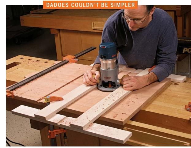
**This is the easy part.** Line up the dado in the fence with your layout lines, clamp the jig in place, and rout. Make multiple light passes for best results, and clamp bookcase sides together to add speed and ensure matching dadoes. For wider dadoes, just move the jig slightly and make another series of passes.
