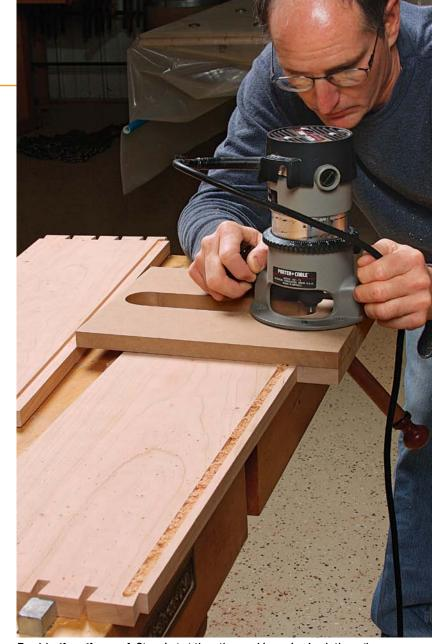
**Rout to the other end.** Stopping at the other end is easier. Look through the viewing window to end right at the layout line.
