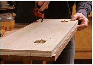
**Setup is simple.** With the hinged section folded down and aligned with the layout line, clamp the back of the jig in place.
