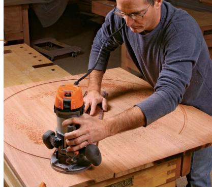
Start with a shallow pass. This lays out the circle for the next step. You'll have to raise the jig and router slightly to get started, unless you are using a plunge router.
