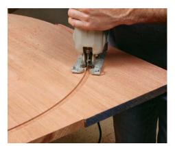
Saw away the waste. A bandsaw will work here, if you can support the workpiece, but a jigsaw is easier. Try to stay within 1/16 in. of the finished edge.
