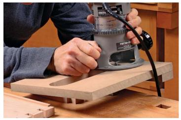
**Watch and tilt.** Turn the router on and look through the jig's viewing window to lower the bit as you begin to move the jig along the edge. Later you can reverse direction to make a clean cut up to your stopping point.
