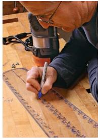
Label it and you're done. After drilling holes to fit the pivot nail, remove the protective paper and use a permanent marker to label each pivot hole. Double-check the distances.
