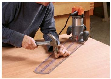
Set the pivot point. Find the approximate center point on the underside of the table, and bang in the pivot nail so it stays tight throughout the cutting process.
