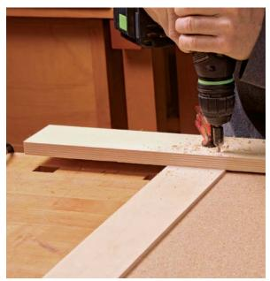
**Attach the second rail.** The spacer ensures that this rail is parallel to and spaced properly from the first one. Again, clamp the fence to the rail before attaching it.
