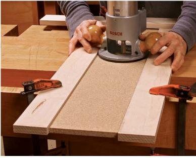
**Spacer aligns the rails.** Rip a spacer just a hair wider than the base of the router, and use it to clamp the second rail in place. The router should slide easily between the rails, but with no slop.
