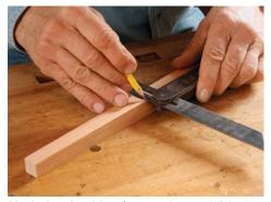
Mark the shoulder. Once you've established the height of the foot, scribe a line around all four sides of the leg. For tapered legs (shown here), you'll need a bevel gauge.
