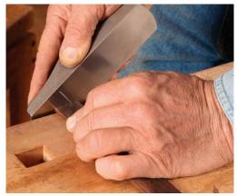
**Bevel the end.** A tapered leg will have an angled shoulder, so you need to angle the foot piece to match
