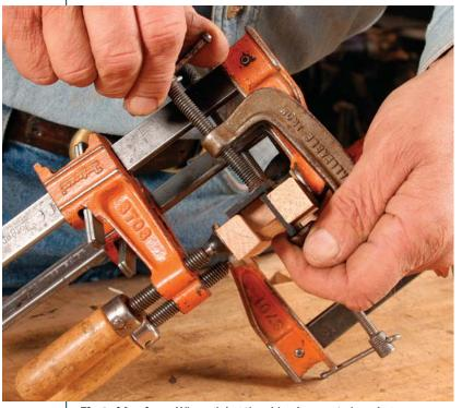
**First side piece.** When gluing the side piece, put clamping pressure against the leg and against the front piece. Cauls make it easier to get the clamps around the inlay pieces.
