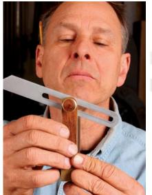
Eyeball it. As you plane the inlay, use the bevel-gauge setting to check the angles on the ends.
