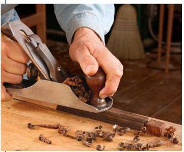
**Pedicure.** Plane the foot flush to the sides of the leg. Then trim the foot pieces flush to the bottom of the leg. Use a block plane to chamfer the corners and the bottom.
