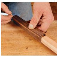
**Back slides home.** Mark the taper on the back piece (above) and plane away material until it slides in from the top without binding (below).
