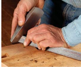
Plane the bevel. Hack uses a handsaw to cut the end of the inlay at the correct angle. Then he adds the bevel using a block plane.
