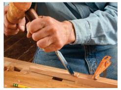
**Clean up the cuts.** Use a handsaw to define the shoulder line, then chop and pare away material to make a clean landing pad for the inlay pieces.
