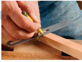
Shoulders are trickier. Set a bevel gauge to the angle, and trace around the leg so that all corners meet perfectly.
