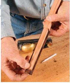
**Slight overhang.** The front piece should project beyond the thickness of the two side pieces.
