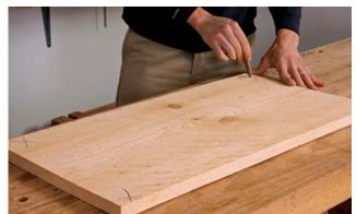
Mark the highs and lows. Using a flat bench or table as a reference surface, find the high and low spots on both sides of the board and mark them with a pencil.
