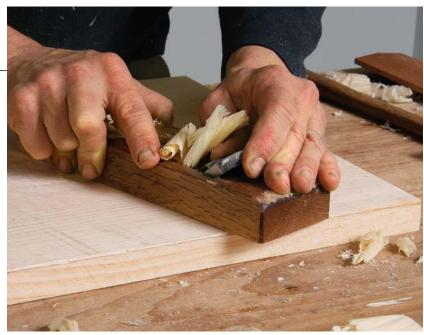
**Second side gets flattened.** Repeat the same sequence of planes and planing angles to flatten the second side and bring the board to the marking gauge lines.
