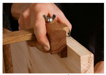
**Leave it a little thick.** Set a marking gauge to  $\frac{1}{16}$  in. over the board's final thickness. Working off the newly flattened surface, scribe a line around the workpiece.
