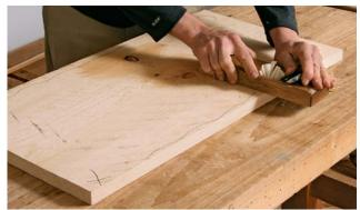
Take out the wobble. Working with a jack plane on the concave side of the board, plane flats along the two long edges until the board, when flipped, lies firmly without rocking.
