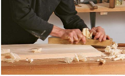
**Along the grain with a longer plane.** After working through the angles with the roughing plane, follow up with a jointer plane. Use the same planing sequence of angled strokes, ending with passes along the grain. Then finish up with a smoothing plane, following the same sequence of strokes.
