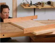
**Check progress with a straightedge.** Using a pencil, Hunter marks high spots with X's and squiggly lines, low spots with O's. Sighting across a pair of winding sticks (right) will tell you if there's any twist in your planed surface.
