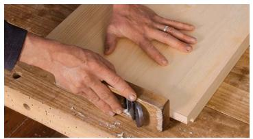
**Shave it to size.** By elevating the workpiece and using your plane on its side, you can use your bench like a shooting board and plane the board to final width (left). After using a knife to lay out the finished length of the board and sawing just shy of the lines, use a jointer plane to trim to the scribe lines (above). To avoid blowing out the grain, take half passes with the plane, shaving from the outside toward the middle.
