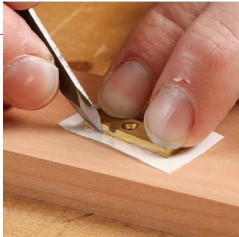
The hinge is its own template. Attach double-sided tape to the bottom of the hinge leaf for secure placement on the workpiece.
