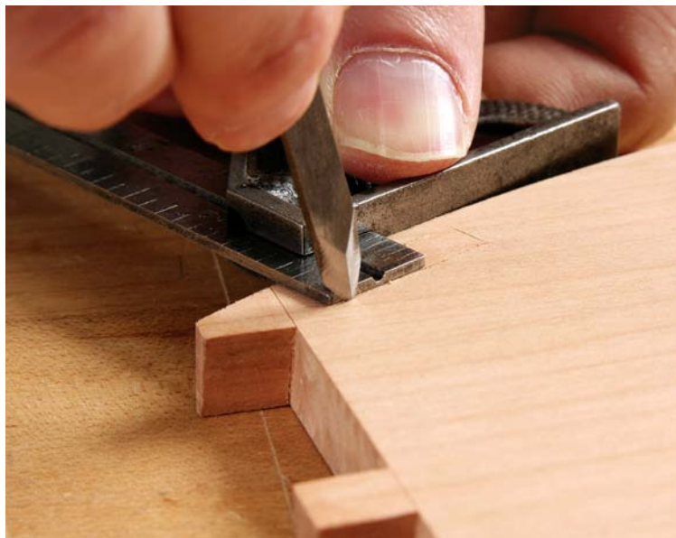
For future reference. Kenney looks down the length of the knife to ensure that its back is parallel to the line. Then he sets the square's blade against the knife, making sure that the end is flat on the knife's back. This distance is crucial; save the setting to use when marking the remaining mortises.
