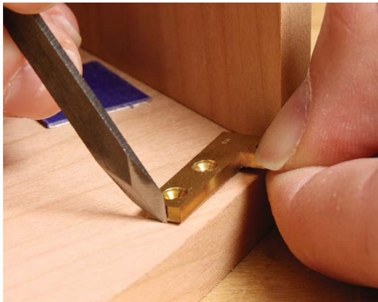
Scribe the layout. Use a knife to scribe around the hinge. Keep the flat face of the knife tight against the hinge.
