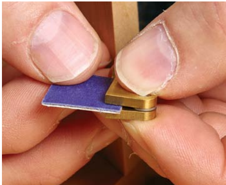
Make a shim. Kenney thickens a business card with blue tape to match the thickness of the washer that goes between hinge leaves.
