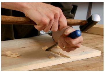
**Rough removal.** Working toward himself with the bevel down, Hunter chisels out all the waste, first on one side of the central relief cut, then on the other.
