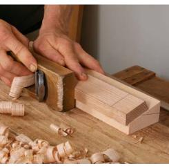
Drive it home. Adjust the fit of the cleat until you can drive it in with moderate hammer blows. Wax helps. Leave a ¼-in. gap at the front end of the socket to allow for seasonal movement of the lid.
