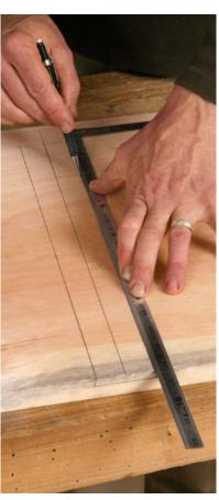
**Cleats fit in a dovetailed socket.** The socket, tapered slightly along its length, is <sup>1</sup>/16 in. wider at the back of the lid than the front.
