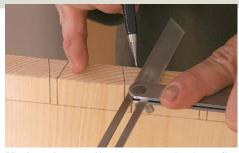
**Mark and score.** Hunter lays out the dovetail pins with a mechanical pencil and a sliding bevel, then scores along the baseline, in the waste areas only, with a marking gauge (right).
