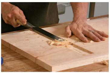
**Out comes the long chisel.** Hunter flattens the bottom of the cleat socket with a long, wide paring chisel. He checks his progress with a straightedge.
