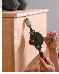
**Drill for the hinges.** Snipe hinges—two linked cotter pins—suit this chest. With the lid weighted, drill an angled hole up through the cleat and lid. Then remove the lid and drill the other hole through the back of the chest.
