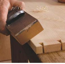
**Final touches before assembly.** With all the joinery cut, Hunter creates a glassy finished surface with light passes of a Japanese smoothing plane (left) and chamfers all exposed edges.
