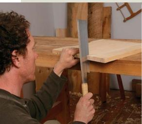
**Rip the pins.** Hunter saws just shy of his layout line, then pares right to it, leaving the line for reference.
