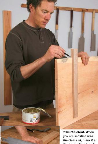
you are satisfied with the cleat's fit, mark it at the back edge of the lid and cut it to length. Then remove it and cut a notch (inset) so the last section lies flush with the lid.
