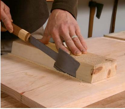
**Automatic angle.** A block of scrap cut to a 14° angle guides the saw to cut the dovetail socket. Hunter draws a line on the sawblade with an erasable marker to gauge the depth of cut.
