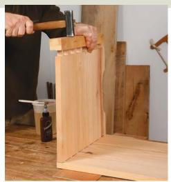
**Knock home the ends.** After applying hide glue to the cheeks of the pins, Hunter hammers home the joint. Then he installs the bottom boards. Scraps of <sup>1</sup>/<sub>4</sub>-in. plywood under the case accommodate the through-dovetails.
