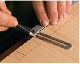
I made the template for just half the opening and used it to lay out both sides. I cut out the curves with a bowsaw and followed it up with spokeshaves and chisels to smooth the cut and fair the curves. You could use a coping saw, or even make multiple relief cuts with a handsaw and chisel away the waste. The best tool is the one you have—making do goes along with the country theme.
