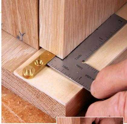
Locate the hinge on the template. Place the template flush with the front edge and ends of the cabinet. Then set the door in place, with the ½2-in. gap behind it. Center the hinge on the thickness of the door and measure the distance to the front edge of the template (above). Then slide the hinge sideways into its true position, and mark the ends of the slot needed in the template (right).
