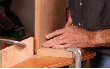
**Rout the mortise.** Stowe uses a featherboard to keep the door tight against the fence.
