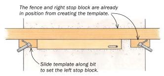
**Clamp on the second block.** With the router off and the bit against the right end of the template mortise, clamp a stop block on the left end of the template.
