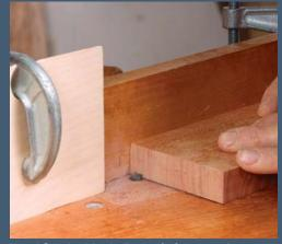
**Head for the block.** For half of the mortises, you'll be able to simply rout into the open end of the mortise until you hit the block.
