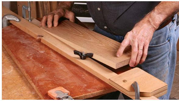
**Rout the top and bottom.** Start with the right end of the workpiece against the stop block. Then lower it onto the spinning bit—being careful to keep it against the fence—and slide it to the other stop block.
