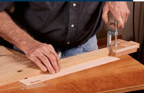
**Reset the stops.** The critical step here is to make sure the bit's cutter is touching the very end of the mortise when you set the stops; otherwise, the mortises in the cabinet won't match each other.
