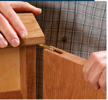
**Slide the door onto the hinges.** The hinge leaves are put onto the hinge pin before they're attached to the door. If you attached them to the door first, you couldn't get them both on the pins.
