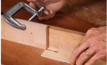
**Set the fence and add a stop.** Use the back edge of the template to reset the fence. You'll be feeding the end of the door directly into the bit, so you need only one stop. This setup routs one mortise in each door.
