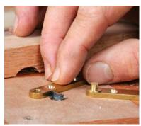
Reset the bit height. It should match the thickness of the hinge leaf exactly, so the leaf ends up flush with the surface.
