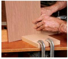
**Move the stop for the next set of mortises.** The stop goes on the right side. The door is dropped onto the bit, then pushed through it.
