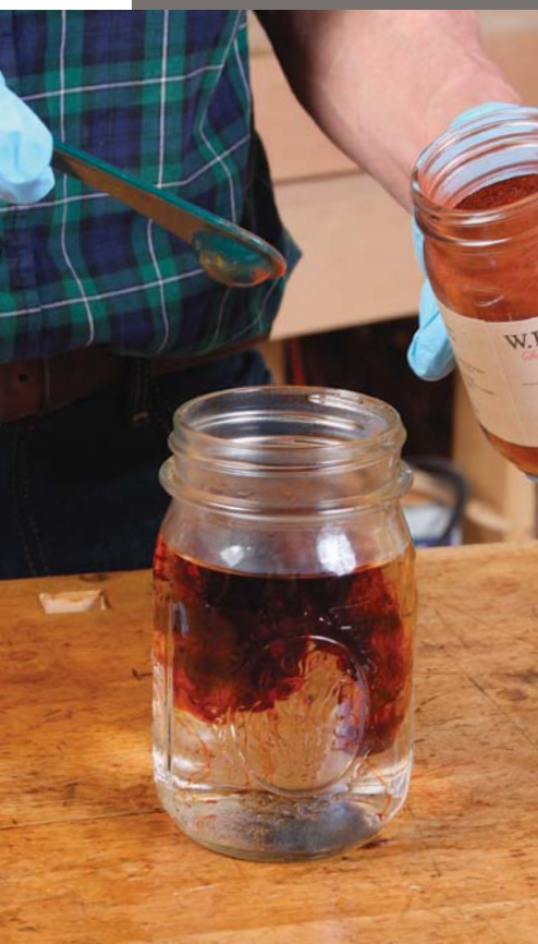
Dye another day. Water-based dyes, once dissolved, will last a year or more if kept in a non-metallic container.
