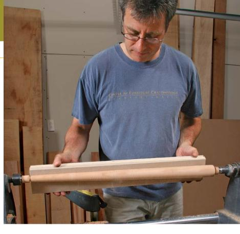
the workpiece. When it came to the legs, I thought turning and tapering them would nicely complement the shape of the top. But wouldn't that make for challenging leg-to-apron joinery? I greatly simplified the matter by dispensing with shouldered tenons and mortising the aprons full-size right into the legs. On a small, light table like this, that would give me plenty of joint strength. To cut the mortises, I built a router jig that took the guesswork out of what might have been a tricky process.
