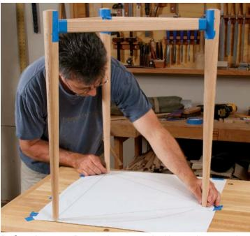
**Perfect placement.** Because there are no shoulders on the aprons, the legs can be adjusted vertically. With the joints just glued, Finan tweaks the legs until they stand within the ¾-in. circles on the drawing.
