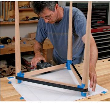
A little belt tightening. After adjusting the stance of the table, Finan cinches up a band clamp. He checks the stance once more and then leaves the table on a flat surface to cure. He will remove the blue tape (which makes glue cleanup easy) before the glue dries.
