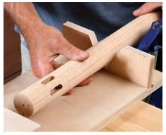
**Plunge with a bushing.** Using a %-in. guide bushing and a %-in. spiral upcut bit in his plunge router, Finan cuts the mortises in a series of progressively deeper passes.
