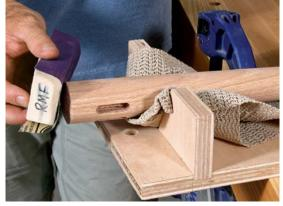
Round the top. After shaping the top of the leg with the parting tool, he sands it smooth.
