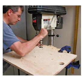
**Drill first, saw later.** Using a Forstner bit, Finan drills the cutouts for the legs at the corners of the top (above). Then it's on to the bandsaw (right) to cut the curved sides of the tabletop.
