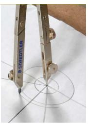
Two compasses create the plan. Finan uses a beam compass (left)—in this case simply a yardstick fitted with a movable pin and pencil—to lay out the curve-sided triangle of the top. He uses a regular compass (above) to establish the circumferences of the legs and the corner cutout of the tabletop.
