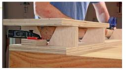
**Snug in the jig.** A clamp at the far end is critical, but the mortise jig is sized so the leg is also held firmly between the routing platform and the cradle blocks. If necessary, Finan unscrews the platform to insert the leg.
