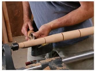
**Tapering tricks.** To achieve a consistent taper, Finan starts by cutting a series of grooves with a parting tool, using his full-scale leg drawing to set his calipers. He uses a roughing gouge (above) to remove the waste between the grooves, then smooths the taper (right) with a long, straight sanding block.
