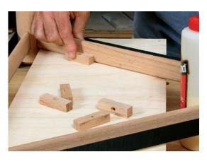
sneak up on a snug fit. After applying glue and getting the pieces knocked together, I stood the base up on the drawing and tweaked the stance until the tips of the legs stood precisely in the small circles. Then I cinched the band clamp, rechecked the stance, and let the glue cure.
