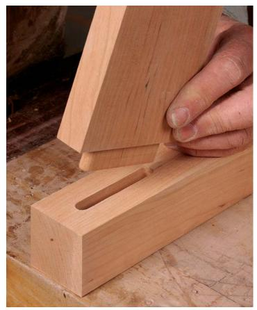
**Dry-fit first.** Then clamp the joint together as tight as it will be after glueup. A tight joint ensures that you'll get wax where you want it (around the joint) but not where you don't (on glue surfaces).
