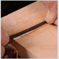
Then glue in the inlay. Use plenty of glue to create a strong bond, and let any squeeze-out dry in a bead, just as you would with a joint.
