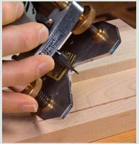
**Spread the wax before routing the grooves.** If you cut the recess first, you're sure to get wax into it and the glue won't bind to the floor and walls of the slot.
