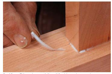
**Peel it up.** This works especially well for drips and runs, as long as you do it about an hour after glue-up, when the glue is firm but still flexible.
