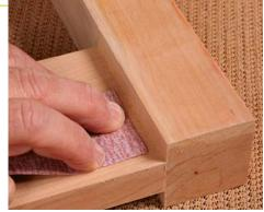
**Sand lightly.** Use P220-grit paper to knock down any grain raised by the denatured alcohol.
