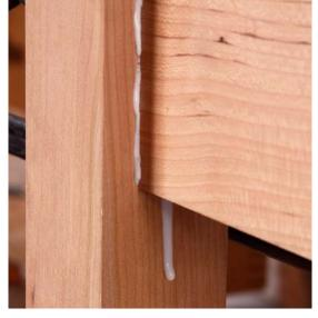
testing with waterborne finishes (which I don't use) and they seem to work fine with the waxes, too. It really is a cure-all for squeeze-out. And the time you spend applying and removing Waxilit is nothing compared to the hassle of removing squeeze-out and then repairing the damage you caused.
