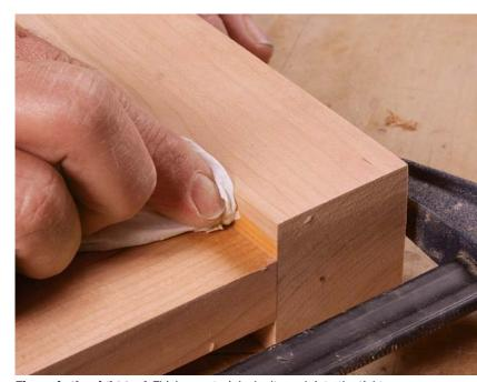
**Tissue is the right tool.** Thicker materials don't reach into the tight corner where parts meet. Apply a thin coat, which should dry clear. If there's a white residue, you've applied too much.
