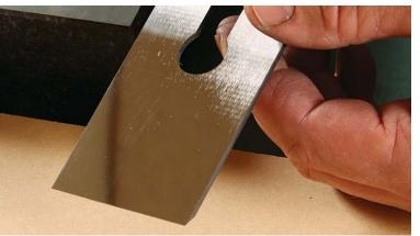
**The payoff.** The back is now ready for work, and you won't need to flatten it again. Removing the burr on the polishing stone (or 2000-grit paper) when you hone the blade is all the maintenance the back needs.
