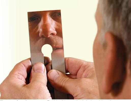
Clear as a mirror, sharp as a razor. The high polish means that the back—and the cutting edge—is truly flat and without blemishes. When it meets a bevel that's just as polished, the blade will be truly sharp.
