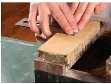
**Use sharpening stones.** Start with a medium grit, like 4000, and finish up with a polishing stone (8000-grit or higher). Make sure the stones are flat before you begin.
