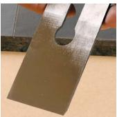
Work up through the grits. On the second grit, move the blade in and out until the side-to-side pattern from the previous grit is gone. Then you can move up to the next grit. Continue to alternate between side-to-side and in-and-out movement as you change grits.
