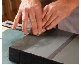
**Or stick with the sandpaper.** Extrafine grits of sandpaper can produce a polish just as well as sharpening stones. A second granite surface plate for polishing is nice, but not necessary.
