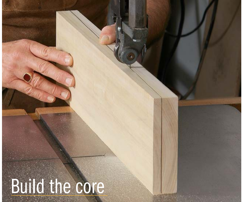
Angled resaw starts the taper. To make the 12-in.-wide tapered core stock, Haig resaws a 6-in.-wide poplar board on a diagonal line. He flips one of the resulting halves end-for-end (so the thick ends correspond) before edge-gluing the pair together.
