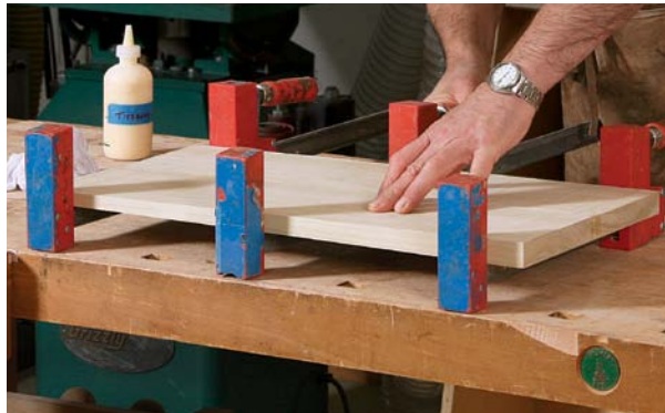
Glued up and tapered off. After gluing up the tapered core (above), Haig smooths the tapered surface with a few passes through a planer on a tapering jig (right).
