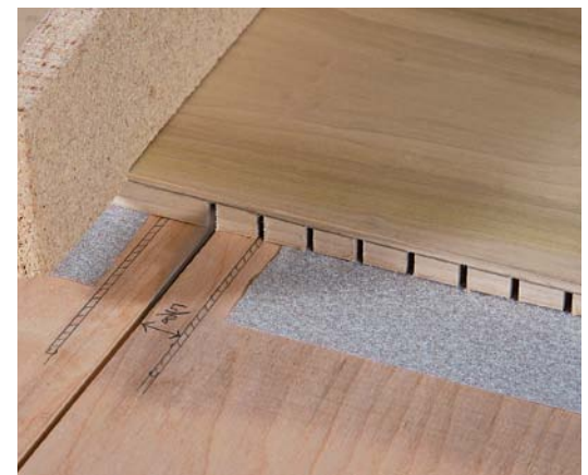
Quick kerfs. Haig cuts kerfs in the core with a purpose-built tablesaw sled and push block (left). Cutting with the workpiece pushed against a front fence enables Haig to use registration lines on the sled to establish quick, accurate spacing between kerfs (above). A pencil line on the workpiece guides the blade height. Sandpaper keeps the workpiece from sliding.
