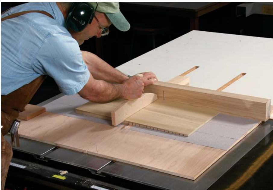
Glued up and tapered off. After gluing up the tapered core (above), Haig smooths the tapered surface with a few passes through a planer on a tapering jig (right).
