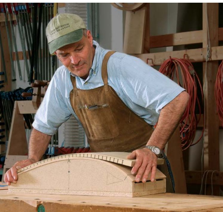
Pliable panels. A solid-wood core kerfed across its width is the heart of Haig's system for making curved, tapered panels. He encases the core in face veneers and steam-bent edging, creating curved panels that look and act like solid wood.
