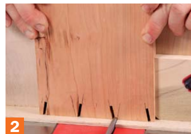
The mirror effect. As you work across the board, moving the board (and stop block) to a new layout line and making all four cuts each time, you naturally begin to cut the second side of every tail.
