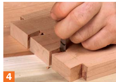
Clean out the waste. After defining all of the tails at the tablesaw, cleanup goes quickly. Work to your scribe lines.
