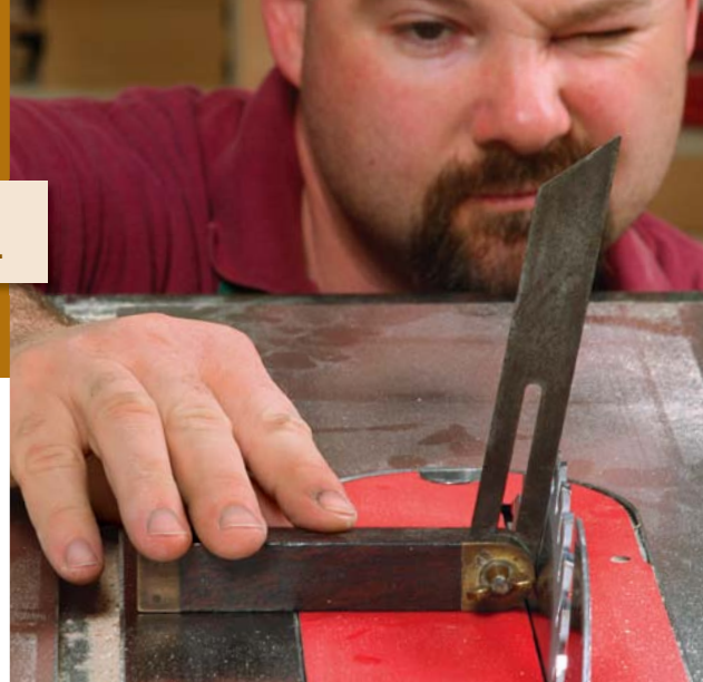
Angle the blade. Make sure the bevel gauge's setting hasn't changed and that it's flat against the blade's plate, coming up in a gullet between teeth.
