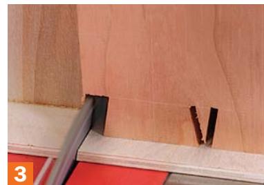
Nibble the ends. A few eyeballed cuts knock off most of the waste at the ends.
