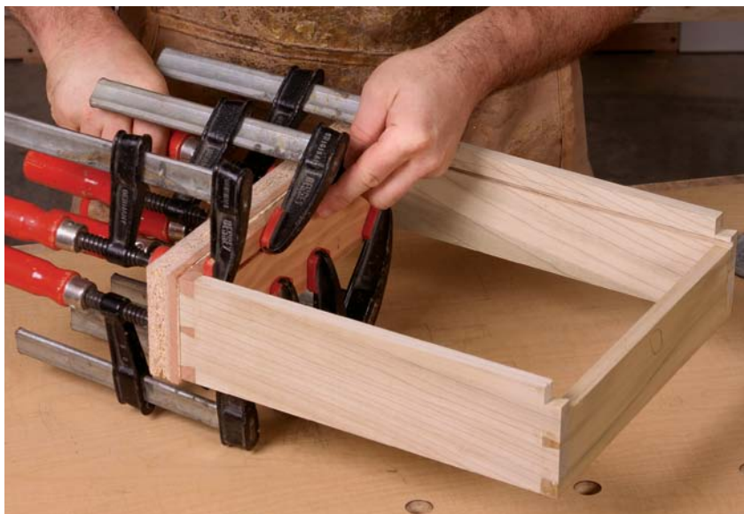
Don't skimp on clamps. Paolini uses a caul made from melamine-covered particle-board to protect the front and help spread the pressure over the entire surface (for a tight glueline around all four sides).
