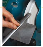
Press in the middle. Keep the gouge tight against the rest and swing the handle to the left and right to create a curved edge.
