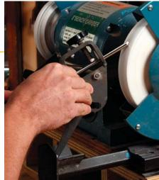
Leg in the pocket. Adjust the pocket of the Oneway jig to set the bevel angle, and grind with no worries.
