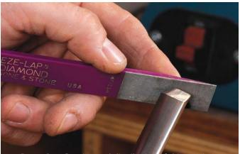
Then the bevel. After regrinding, brace the tool against the rest or a workbench and hone the beveled edge with a diamond paddle.
