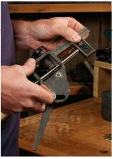
Set the projection. Adjust the gouge so that it sticks out about 2 in. from the Vari-Grind jig.
