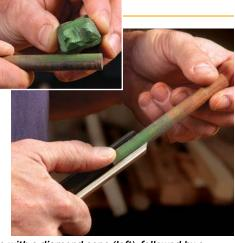
**Inside first.** Hone the first  $\frac{1}{2}$  in. of the gouge's flute with a diamond cone (left), followed by a dowel charged with jeweler's rouge or finer-grit buffing compound (right). Keep both flat in the flute to avoid beveling the edge.
