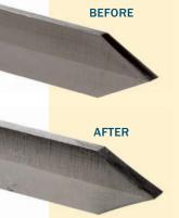
Straight out of the package, the diamond parting tool needs just a quick touch-up on the bench grinder. It's the only tool that needn't be honed.
