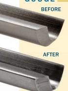
New gouges have bevels that are too steep and short for effective turning. Regrind them to lengthen the bevel, and then hone the edge.
