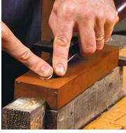
Hone on stones. Rock the hollowground bevel to find the flat spot and then drag it in a sweeping motion to hone the edges.
