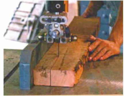
The right blade for hardwoods. Ripping hardwoods on the bandsaw is easy with a \frac{1}{2} -in.-wide, 4-pitch blade.
