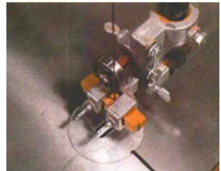
Tight curves, clean cuts. A \frac{1}{16} -in., 24-pitch blade cuts intricate scrolls with little or no cleanup required.
