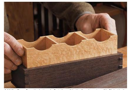
**Add the liner.** Drop the bottom in first, then slide the liner in on top of it. Gluing isn't necessary. The portion of the liner that extends above the box sides may need to be beveled slightly on the outside faces to allow the lid to lift off easily.
