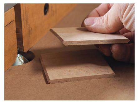
**Dividers get beveled ends.** Set the chamfer bit to cut a bevel half the thickness of the stock. Flip the divider to cut the second bevel.
