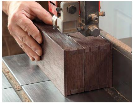
**Slice off the lid.** After gluing up the box, cut it in two at the bandsaw. Center the kerf in the middle of the wider dovetail. Chamfer the edges of the cut, but leave the bandsaw marks and burnish them with steel wool.
