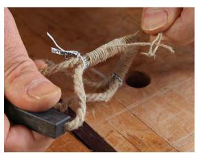
Add a wrap to the cord. Use thinner twine to wrap the cords between the twist ties. Start with a few wraps over the end of the twine to secure the starting end of the wrap. Before reaching the opposite tie, insert a loop of twine under the wrap (top). When you reach the end, thread the twine through the loop and pull it to draw the end under the wrap (above).
