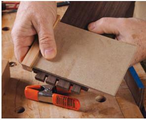
A little help with the dovetails. A simple shoulder guide positioned along the baseline (above) and held in place with a spring clamp helps ensure proper alignment of the parts for scribing (right). Adding tape to the end grain and peeling away the waste after scribing offers a clear road map for sawing (below).
