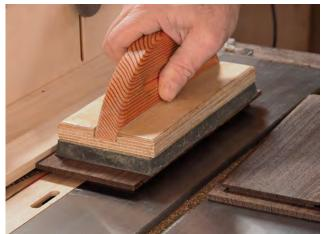
Trim the top and bottom. Rip along the edges of the top and bottom to create a short tongue and allow the lip to overhang the sides. The ends of the box are not grooved, so turn the grooves at the ends of the top and bottom into rabbets.
