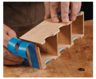
Wrap it up. After cutting the scallops in the sides, lay the liner parts facedown on the bench and apply tape across the joints. Flip them over and add glue to the miters and V-grooves, then roll up the assembly. The tape should be enough to keep the miters tight, but clamps may need to be added across the dividers to tighten gaps at the V-grooves.
