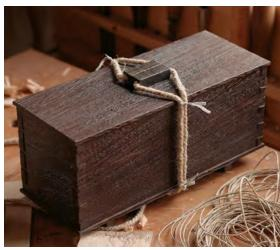
**String it up.** Loop the cord through the holes in the base and clasp. Add a twist tie at the top and bottom edge of each side. Adjust as necessary until the clasp is centered on the lid (above), then drive and glue a wedged dowel into the oval hole in the base that the cord ends are threaded through (right).
