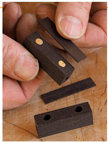
**Add magnets and cap it with veneer.** For extra strength, drop a pair of magnets into each hole. Double-check their orientation to make sure the halves attract instead of repel each other. Then cap the magnets with a thin strip of ebony. If the cap is too thick it will reduce the attraction of the magnets.
