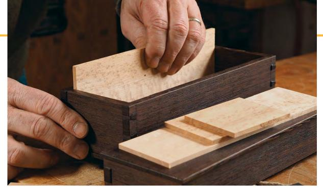
V-grooves, then miters. The liner joinery can be handled at the router table. Start by cutting the V-grooves while the ends of the stock are still square (right). Then set a chamfer bit to cut a miter almost the full thickness of the stock (far right). Leave a small flat at the top to ensure that the liner is not shortened during mitering.
