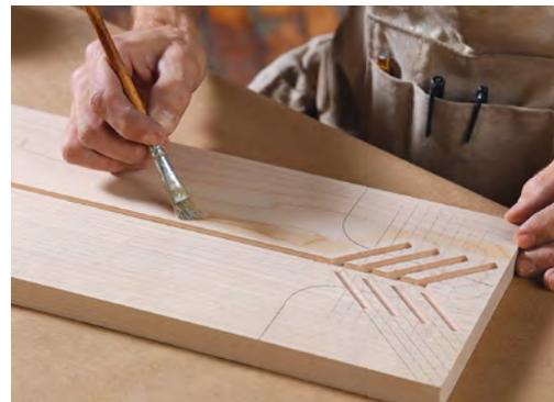
**Build a dam.** Brush on a strip of furniture wax about  $\frac{1}{4}$  in. from the groove, following the contour of the overall design but not dipping between close-set grooves (top). Next, lay down a bead of pure silicone caulk, like GE Type 1, in the middle of the wax. Blue tape, when pressed firmly to the wood, makes a good dam at the ends of grooves that run out the board's edge (bottom). Wait for the caulk to dry before pouring the epoxy.
