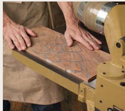
**Remove the waste.** After filling the grooves with epoxy and flushing it off, Moore runs the blank through his planer to remove the bottom (take light cuts), exposing the epoxy inlay on both the top and underside.
