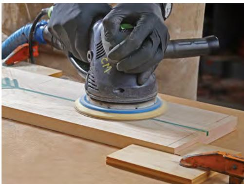
**Rough out the shape.** Cut close to the layout lines drawn on the blank before the grooves were routed.
