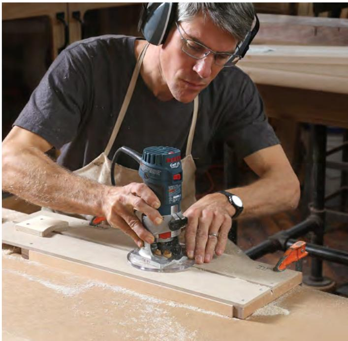
**Rout the grooves.** Because the epoxy is translucent, the grooves must be cut cleanly without burning, so use a sharp bit in the router.
