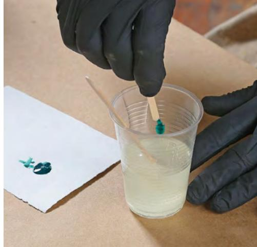
**Tint and fill.** Using a toothpick or a small stick, add one drop of pigment at a time (top). Mix with a tongue depressor. After you've gotten the color right, pour the epoxy into a second cup (bottom). Don't scrape out the first cup; you want unmixed parts to stay behind in the original cup.
