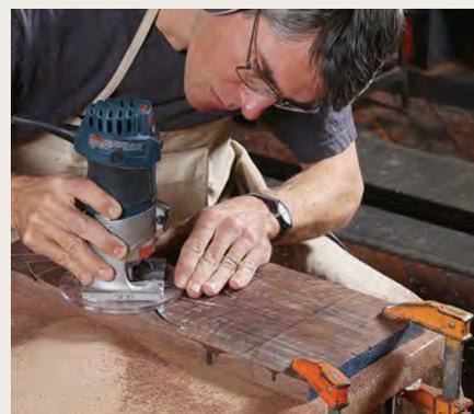
**Deep grooves.** Start by cutting deep grooves in an overthick blank. For some patterns Moore works without a template. After drawing the design on the blank, he follows the lines freehand, moving slowly to control the router.
