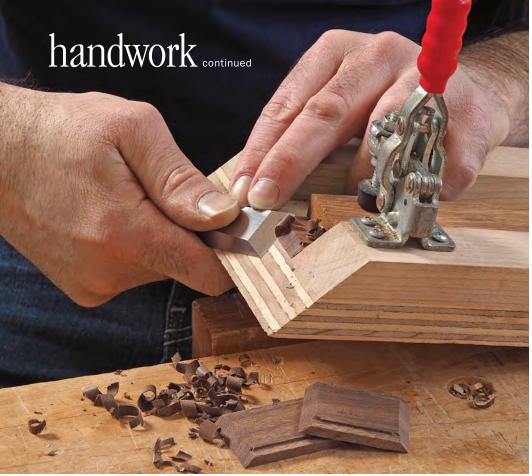
**Cut small miters.** Kenney makes very small boxes. Some have sides just  $\frac{3}{16}$  in. thick, and  $\frac{1}{2}$  in. wide and long. That's too small to miter with a tablesaw, but a wide chisel and an accurate jig allow him to cut the miter very quickly. The smooth surface left by the chisel results in a joint so tight it disappears.
