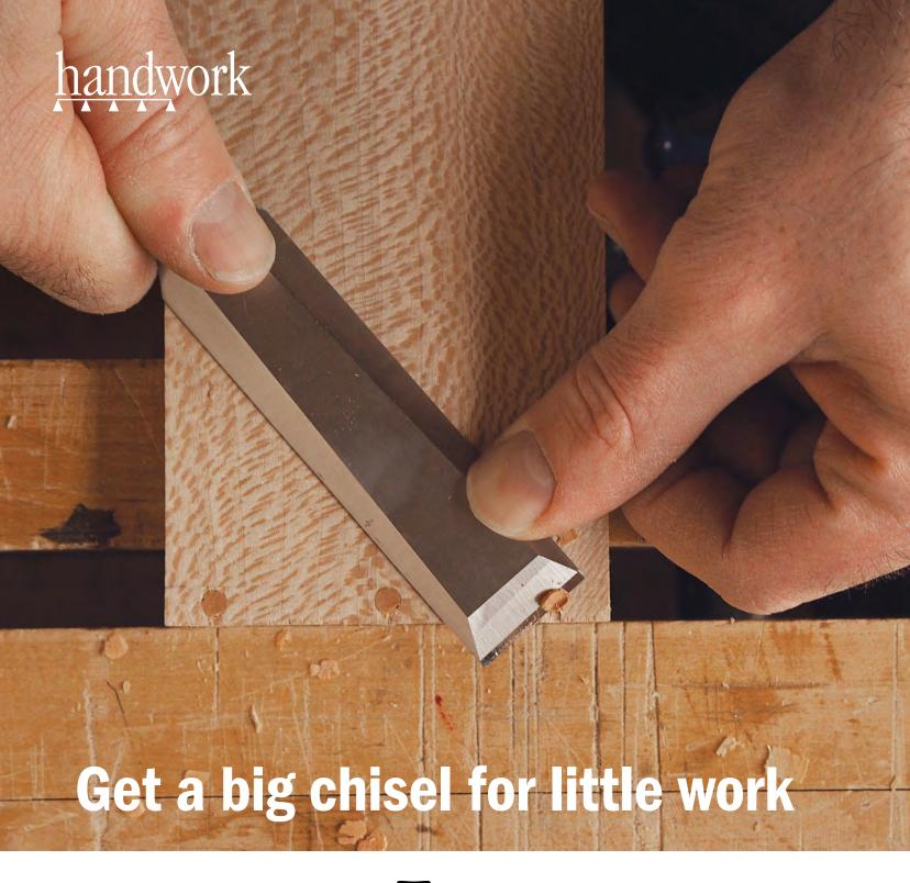
A 1-IN. CHISEL IS A GREAT CHOICE FOR PARING AND CUTTING SMALL-SCALE JOINERY
