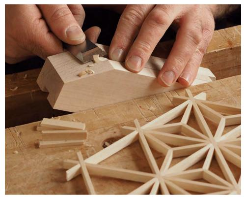
**Quick kumiko.** The tiny pieces that fit together to create patterns inside a kumiko frame must have dead-accurate angles cut on their ends. A sharp, wide chisel can cut these angles very quickly and accurately. The key is to keep the chisel's back flat on the paring guide for the final pass.
