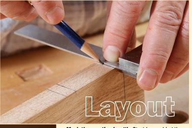
Mark the mortise length. Start by marking the rail width on the stile, then measure in \(^3\)/8 in. to locate the mortise ends.
