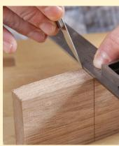
Lay out the tenon shoulders. The length of the tenon should equal the width of the stile. Use a knife and square to wrap the shoulder line around the piece.
