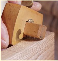
**Scribe the mortise walls.** Run the gauge between the end lines of the mortise on each edge of the stock. Make sure to reference off the show face.
