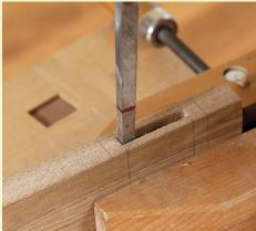
Lever and repeat. Lever the waste, and move the chisel ½ in. farther. Chop and lever again. When you lever, make sure the fibers are free to move. At the ends of the mortise, rotate the chisel so the bevel is facing inward.
