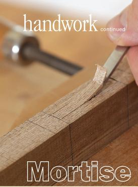
Make a space for your chisel. Starting on the inside edge, make stop cuts with a chisel at the ends of the mortise. With the chisel bevel down, lift out a shaving between the cuts. This groove helps precisely register your chisel.
