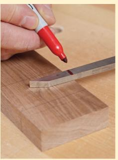
**Draw your depth gauge.** To monitor the depth of cut, draw a mark around the chisel representing slightly more than half the width of the stile.
