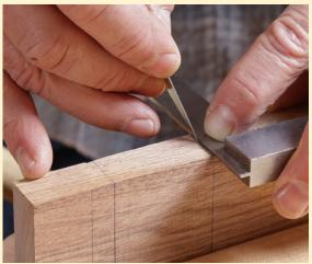
Knife the mortise ends. With the mortise walls scribed, knife the mortise ends along the pencil lines, starting and stopping at each scribe line. The knifed line will register your chisel when you chop.
