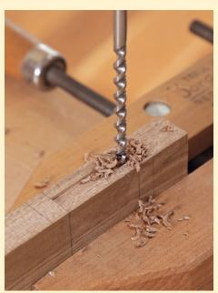
**Drill a starter hole.** Bore a <sup>1</sup>/<sub>4</sub>-in.-dia. hole halfway through the stile near the mortise end closer to you. This hole enables the chisel to plunge deeply right off the bat.
