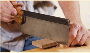
**Cut the shoulder.** Place a saw into the bevel and butt the saw teeth against the tenon shoulder. Next, with a steady hand, cut the shoulder down to the cheek. Repeat on the other side.
