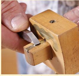
**Set the mortise gauge using the chisel.** Adjust the pins so the <sup>1</sup>/<sub>4</sub>-in. chisel drops just inside them. Keep this setting for the whole process. Set the fence to center the mortise on the stock.
