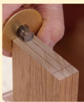
Scribe the tenon's width. Mark % in. from both edges. Scribe the ends only. After you cut the cheeks, bring these marks down the tenon.
