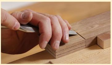
**Define the shoulder.** Use a 1-in. paring chisel to cut a bevel on the waste side of the knifed shoulder lines.
