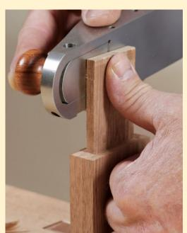
Fit the joint. Spread pencil lead on the mortise walls and then assemble the joint as far as you can. Remove the tenon: graphite will be on the tight spots. High spots inside the mortise may also be burnished. Remove these with a chisel or plane until the fit is right. If the pieces are out of square, relieve the areas pushing the joint out of alignment.
