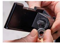
Big and adjustable. The Craftsman (shown here) has the biggest tool-rest platforms. Both it and the Porter-Cable are easily adjusted. Unfortunately, each one has detents in the adjustment mechanism that limit the angle settings. A simple fix is to place a washer spacer over the detents (above).
