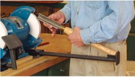
Easy upgrades. The best solution to a faulty tool rest is to invest in an aftermarket model, such as the Veritas (left, \$50), which took Best Overall and Best Value in a head-to-head comparison (FWW #174). Another option is the Wolverine jig (above, \$88), which comes with both a flat rest and a clever arm for turning tools.
