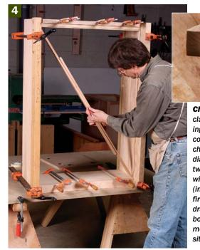
Check inside. If clamps are blocking the outside corners, you can check the interior diagonals using two sliding sticks with pointed ends (inset). Measure the first diagonal and draw a line across both sticks. Then measure the opposite diagonal.
