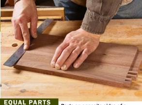
Parts on opposite sides of a piece must be the same length between shoulders to ensure square corners.
