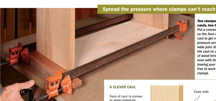
Two clamps, two cauls, two hands. Put a convex curve on the face of a caul to get even pressure across a wide joint. Elevating the caul on a block of wood brings it even with the joint, leaving your hands free to work the clamps.
