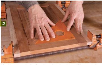
**Flexible choice.** A raised panel may interfere with a rigid square but a plastic triangle can be bent downward to contact the frame.
