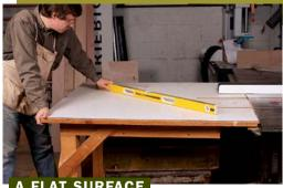
Use a 4-ft. level to see if your bench or outfeed table (above) is flat. If it isn't, clamp a piece of 3/4-in.-thick MDF or plywood to a pair of sawhorses and use shims to bring that surface flat (right).
