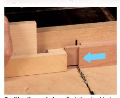
**Position the workpiece.** Push the stop block toward the blade, and the workpiece toward the block.
