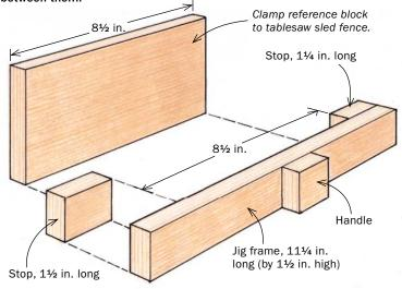
All parts made from <sup>1</sup>/<sub>2</sub>-in.-thick plywood.
