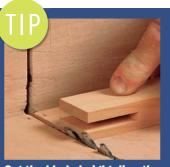
Set the blade height directly from the stile. It's quicker and more reliable than transferring a measurement from the slot.
