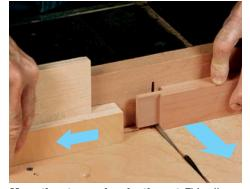
Move the stop and make the cut. This allows the waste piece to move away freely.
