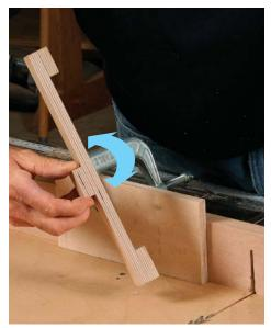
**Flip the stop.** The reference block ensures that it ends up in the right place.
