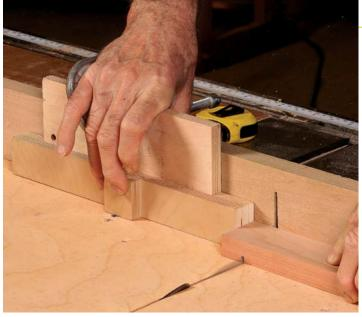
**Cut the short shoulder first.** Use the end with the longer stop to make the shorter side.
