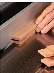
The first one is made with the rails and stiles face down, the second is with them on edge to free the waste.
