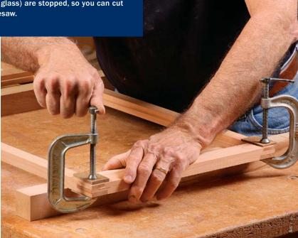
One clamp for each joint. If the frame is square and the joints tight, you don't need clamps across the width and length.
