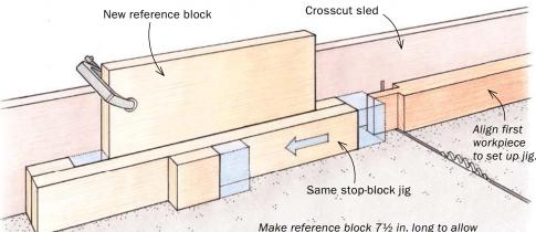
Make reference block  $7\frac{1}{2}$  in. long to allow the stop to slide back from the tenon.
