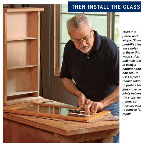
Hold it in place with stops. Stowe predrills clearance holes in these thin wood strips and nails them in using a hammer and nail set. He uses a piece of manila folder to protect the glass. Use butt joints between the stops, not miters, so they are easy to remove for repair.
