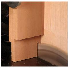
**Use the jig to cut the tenon's width, too.** Set the blade height to the lower (rear) shoulder.
